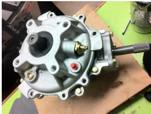
Figure 5: Polaris Ranger rear end locking differential
