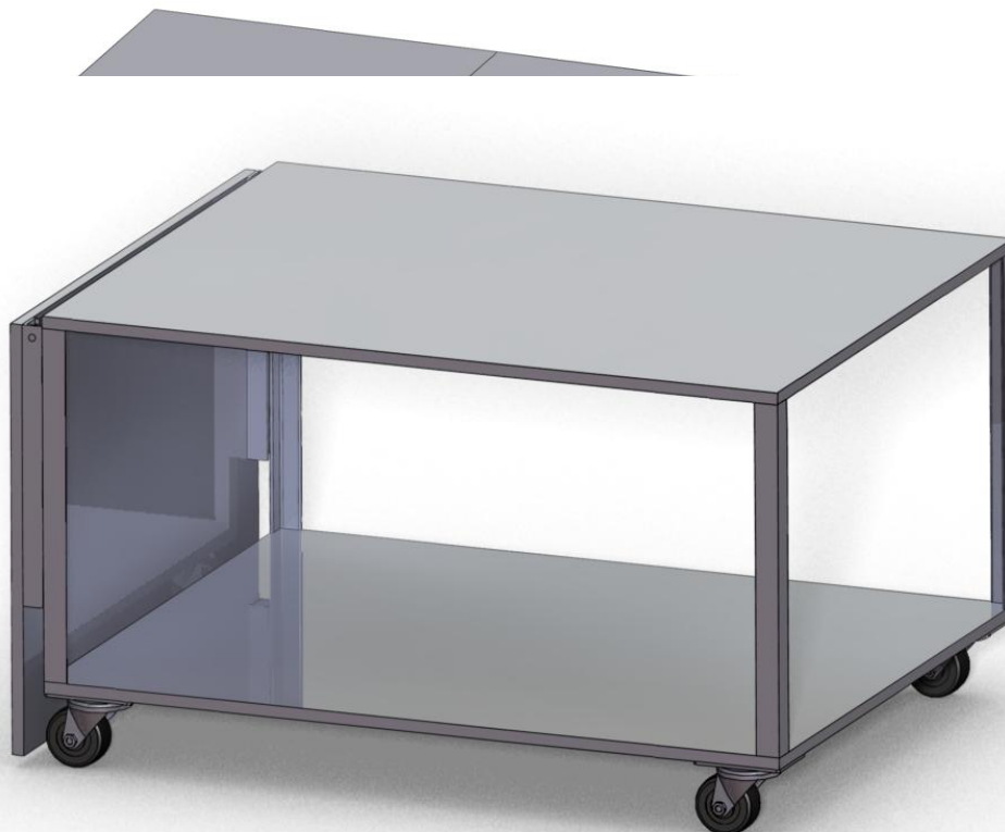
Figure 28. Final Design - Brackets Folded.
