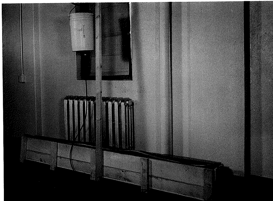
Fig. 4.3 Plastic container with a float valve connected to the test sample
