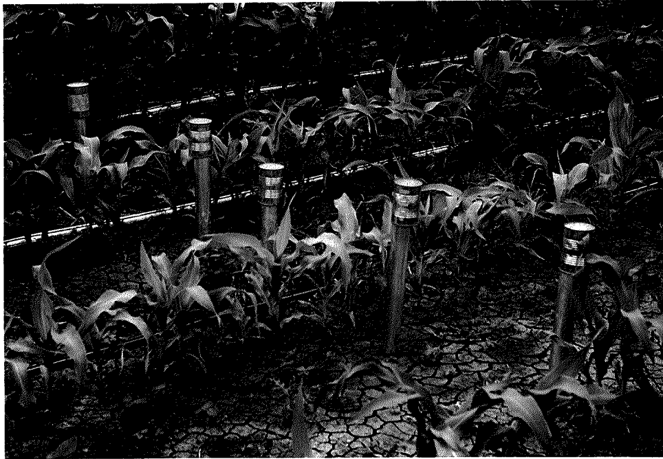
Fig. 4.5 Installation of access tubes at a moisture monitoring station
