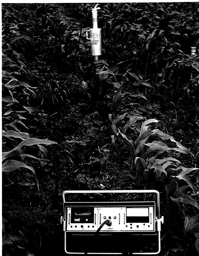
Fig. 4.14 Troxler depth moisture gauge and Troxler ratemeter connected
