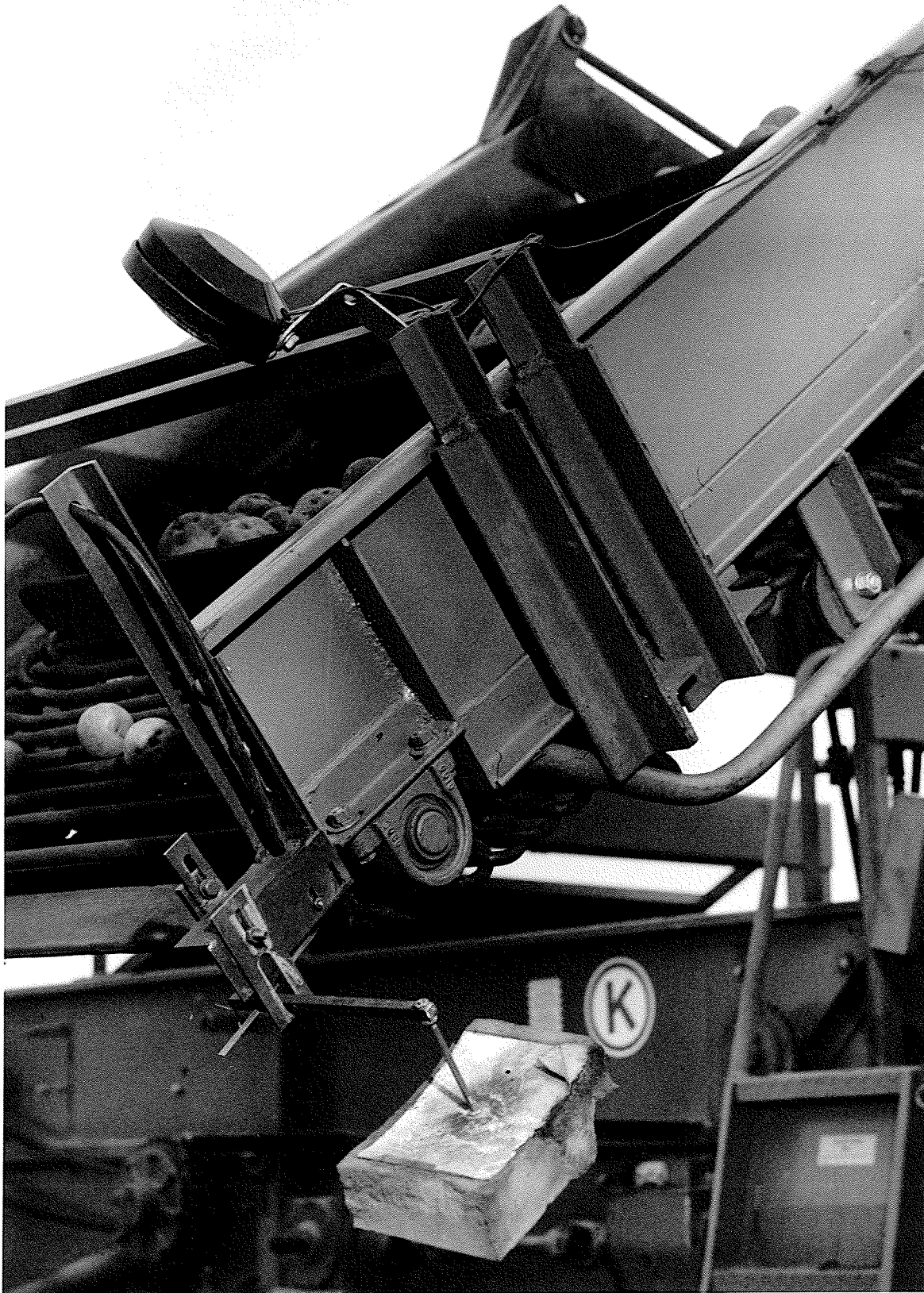
Fig. 6.2 Final Version of Actuating Arm for Activating the Microswitch
