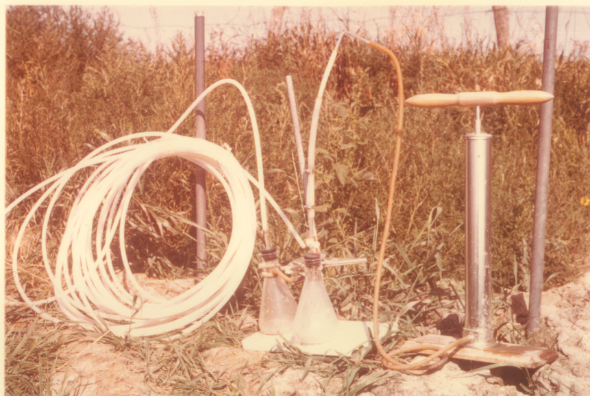
Plate 3 Apparatus used to sample piezometers -Vacuum pump -Vacuum bottle -Tygon tube
