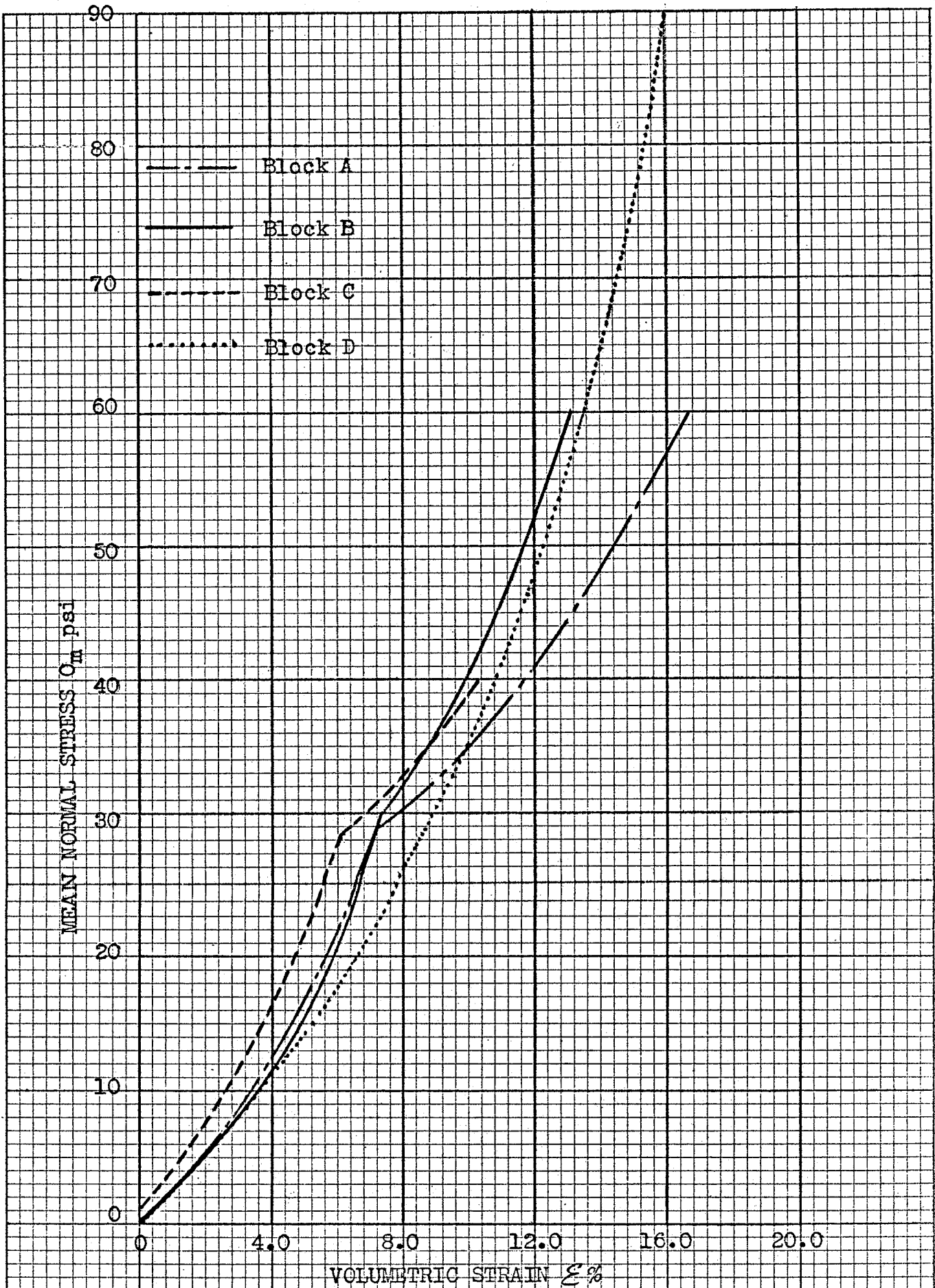
Figure 8. Comparison of Volumetric Stress-Strain Relationships for Blocks A, B, C and D.
