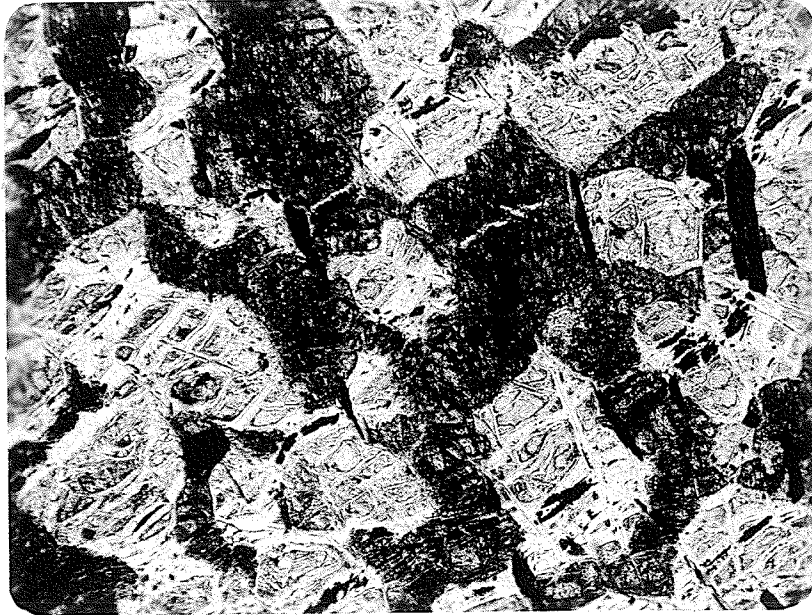
PLATE 13: Poikilitic plate of tremolite (at extinction) pseudomorphic after pyroxene and enclosing serpentine pseudomorphs after olivine. #164. (x42).
