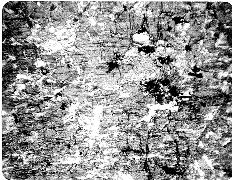
PLATE 8: Orthopyroxene (grey) being replaced by wispy laths of tremolite (white). The replacement is guided, but not completely controlled by the pyroxene cleavage #130. (x34).
