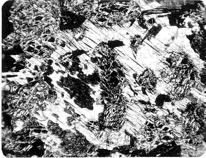
PLATE 21: Poikilitic clinocllore enclosing partially serpentinized olivine, hypersthene and tremolite. #52. (x30).
