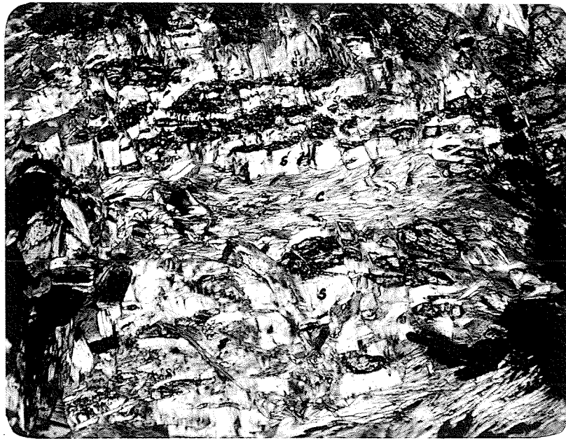
PLATE 6: Regenerated string-like olivine grains (high relief) in serpentine (S). Fine flaky chlorite (C) forms central band. Sulphides (black). #104. (x100).
