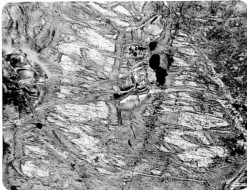
PLATE 10: Highly serpentinized orthopyroxene (white) enclosing serpentine pseudomorph after olivine and a few red spinels. #125. (x115).
