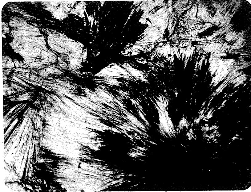
PLATE 17: Fibrous rosette pattern of anthophyllite as developed in a massive specimen from Setting Lake. Fine grained magnetite is also present. #15. (x22).
