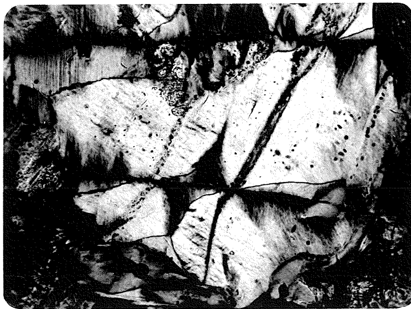
PLATE 33: Leaf-shaped arrangement of fibrous chrysotile. All fibers have negative elongation. Fine magnetite grains are concentrated in the partings. #86. (x272).
