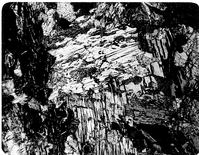
PLATE 20: Clinochlore crystals (CL) surrounding remnant tremolite fragments (T). Narrow lenses carbonate and an opaque oxide occupy the chlorite cleavages. #136. (x40).
