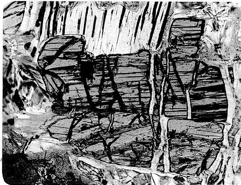
PLATE 16: Twinned tremolite crystal veined by cross-fibre serpentine. Clinocllore (white, at top) is unaffected by the serpentine. #113. (x113).
