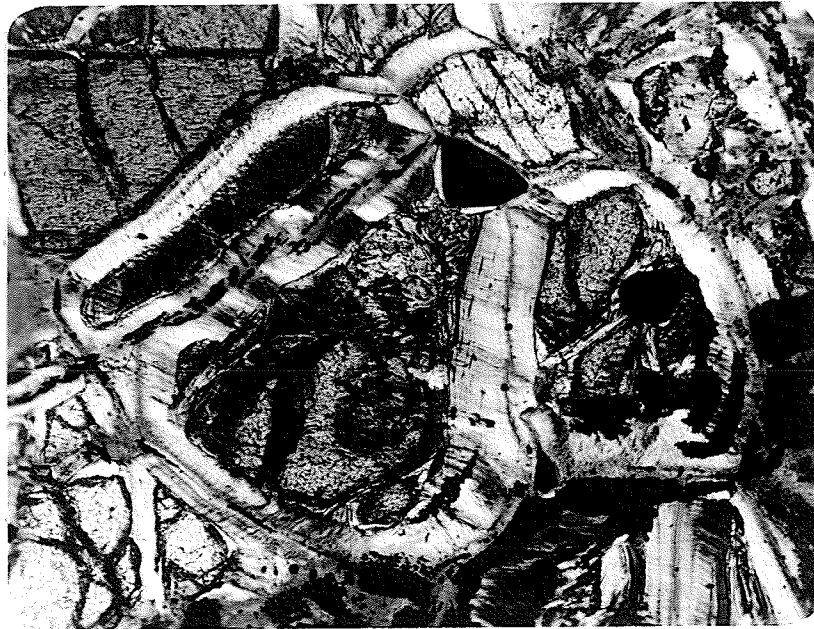
PLATE 27: Fibrous chrysotile veinlets completely surrounding remnant olivine grains which are being further replaced by a greenish-brown serpentine or chlorite. Opaque minerals magnetite. #109. (x107).
