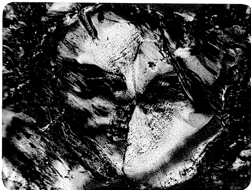
PLATE 35: Segmented arrangement of fibrous chrysotile showing flamboyant extinction. Two of the segments (upper right and lower left) are of \gamma -serpentine with different attitude to remaining \alpha -serpentine. #73. (x160).
