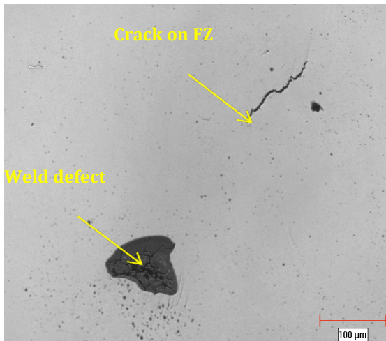
Figure 4.19 R80: Optical, showing weld defect
