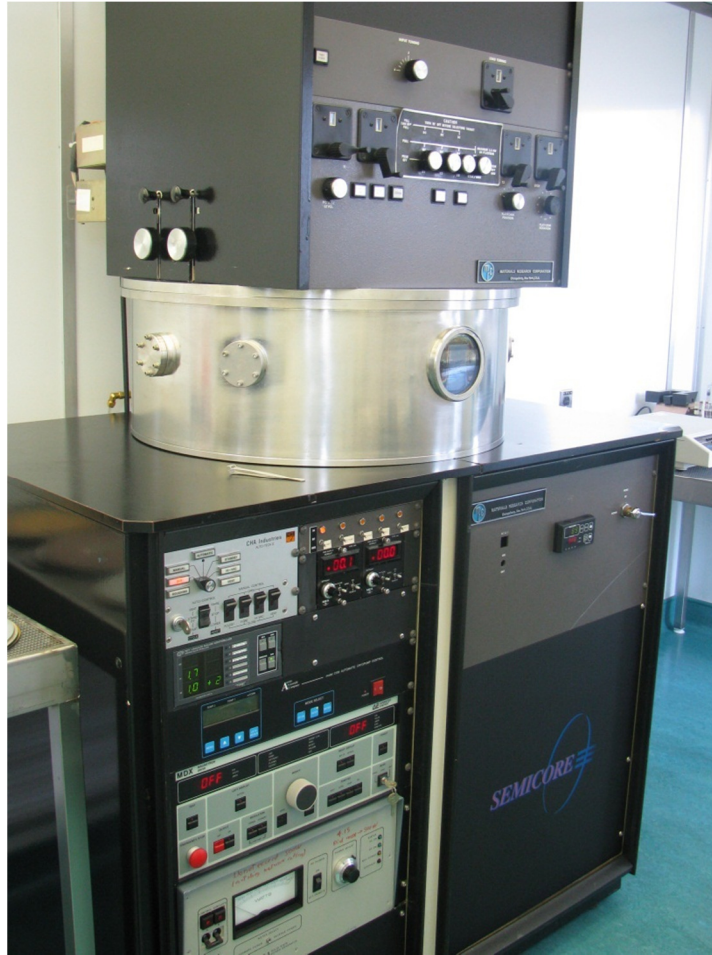
Figure 4: NSFL MRC 8667 sputtering system.
