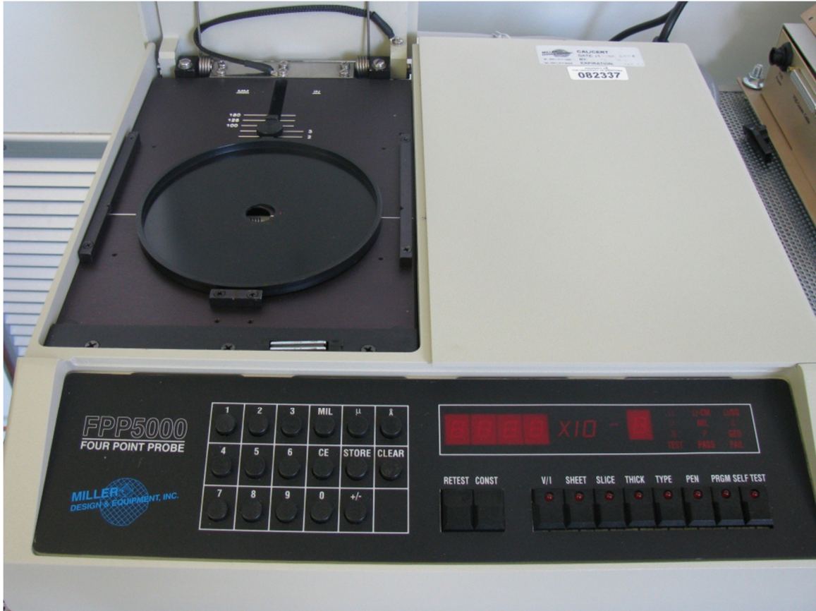
Figure 72: Four-point probe measurement device.
