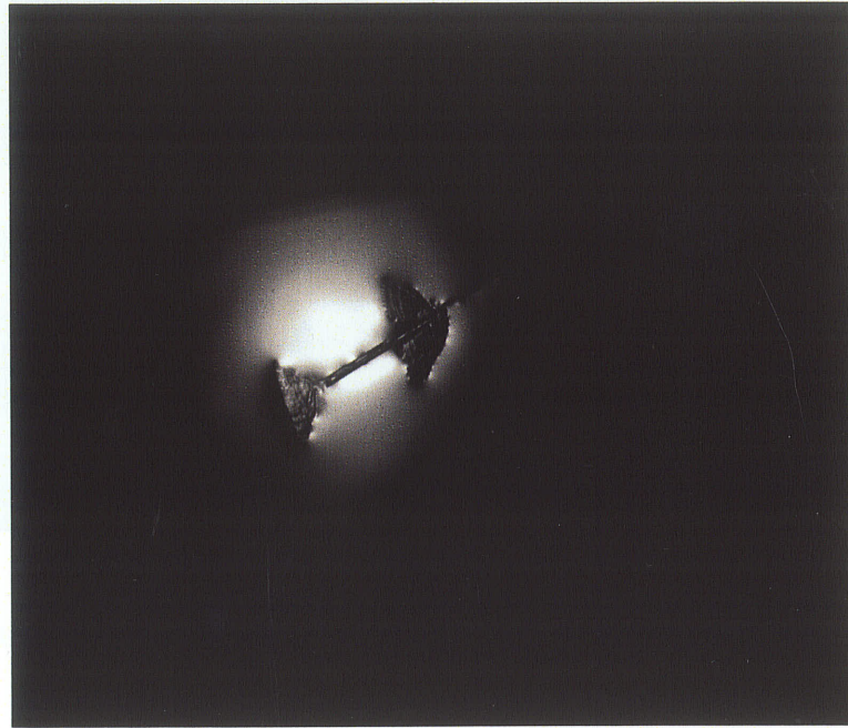
Figure 5.3. Skim ice run (top camera) ( d=10\text{mm} , h=0.15\text{ m} , U=0.2\text{ m/s} and T=-15^\circ\text{C} )
