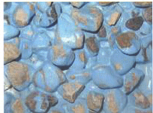
Figure 4.2 Small ( D_{50} = 3.5 mm) and large ( D_{50} = 10 mm) diameter gravel used for the bed plates.
