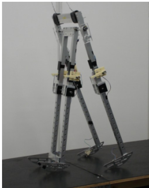
Figure 1.8: Passive dynamic walker with active knee locking mechanism built in Waseda University, Japan
