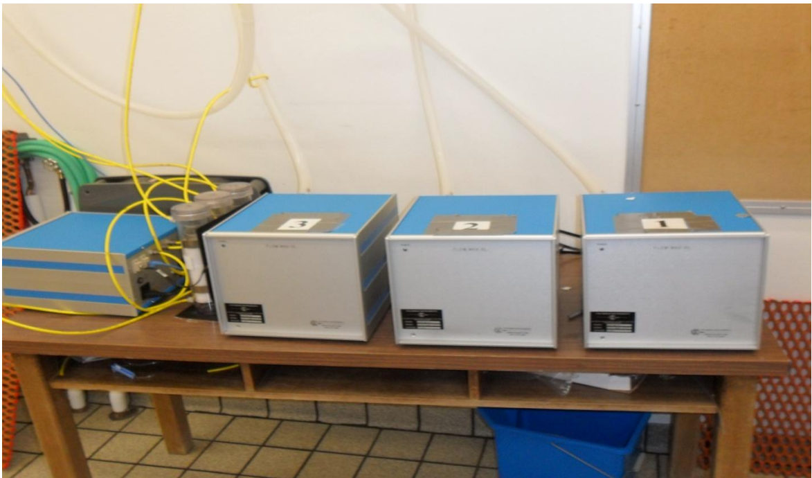
Figure 4.2b. From left: Oxymax sample pump, three (3) gas driers (cylindrical system) and three (3) fresh air blowers ( one per respiratory chamber)
