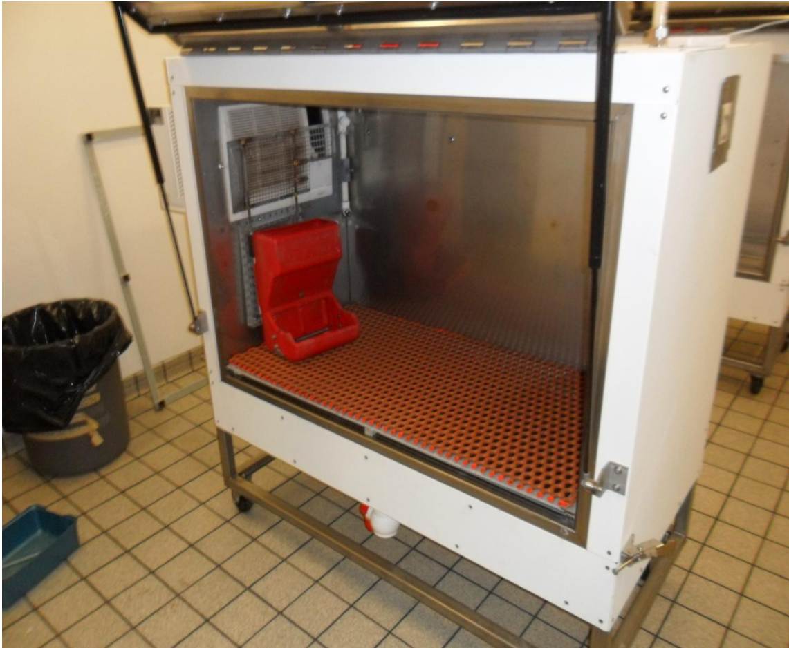
Figure 4.1. The Oxymax open-circuit indirect calorimeter
