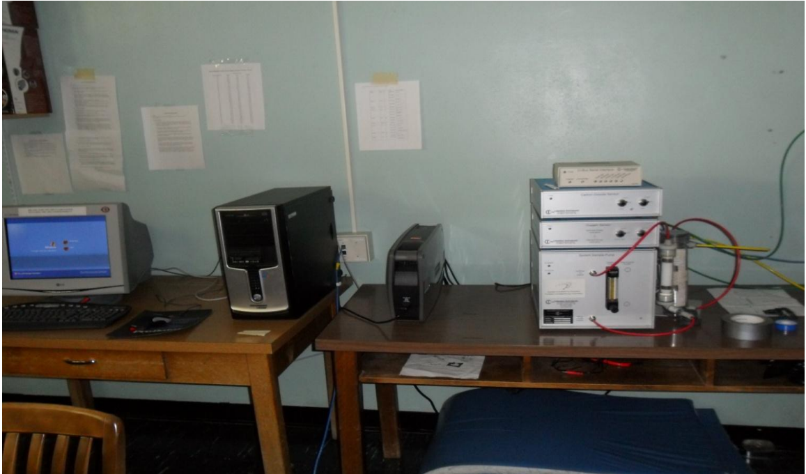
Figure 4.2a. Terminal computer and Oxymax integrated instrumentation with O 2 and CO 2 sensors (extreme right)
