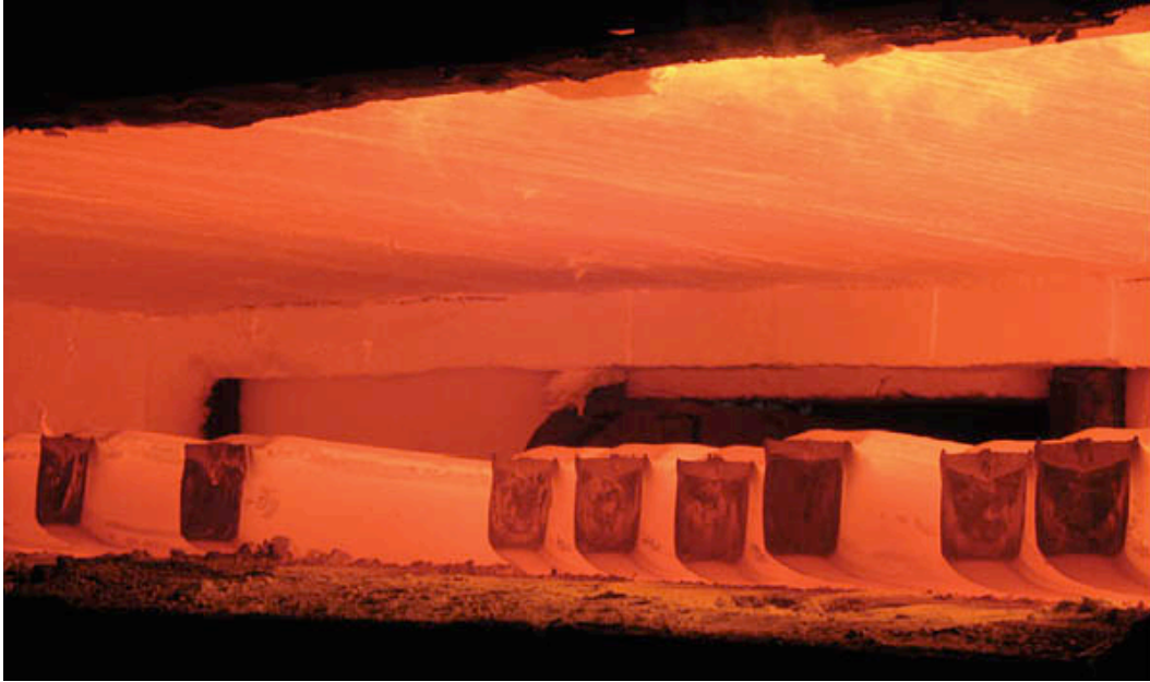
Figure 25: Steel reheating process in the reheat furnace
