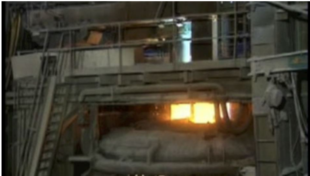
Figure 33: The EBT furnace at Gerdau
