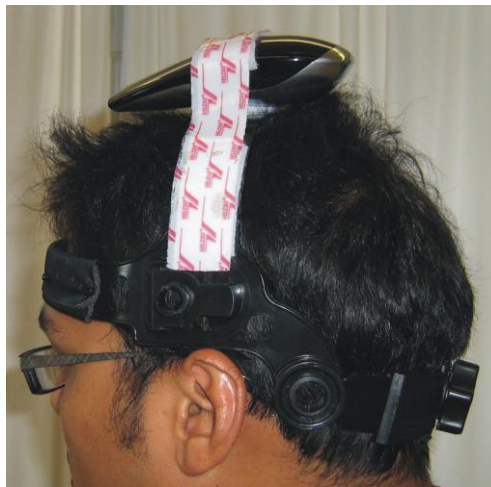
Picture 4. Gyration Air –mouse fitted in helmet.
