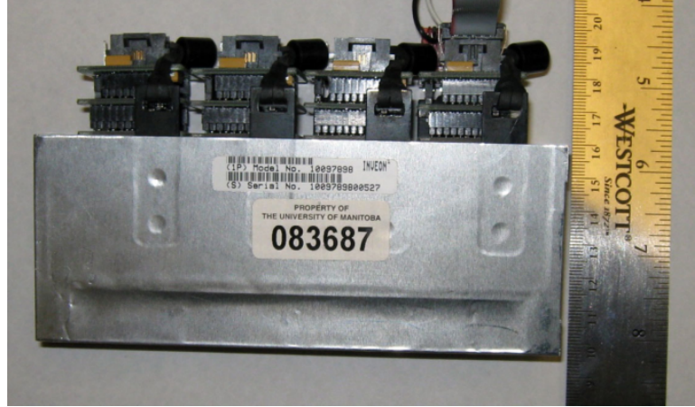
Figure 2.2: Inveon detector module that contains 4 block detectors and their preamplifier stacks in a light-tight aluminum enclosure.
