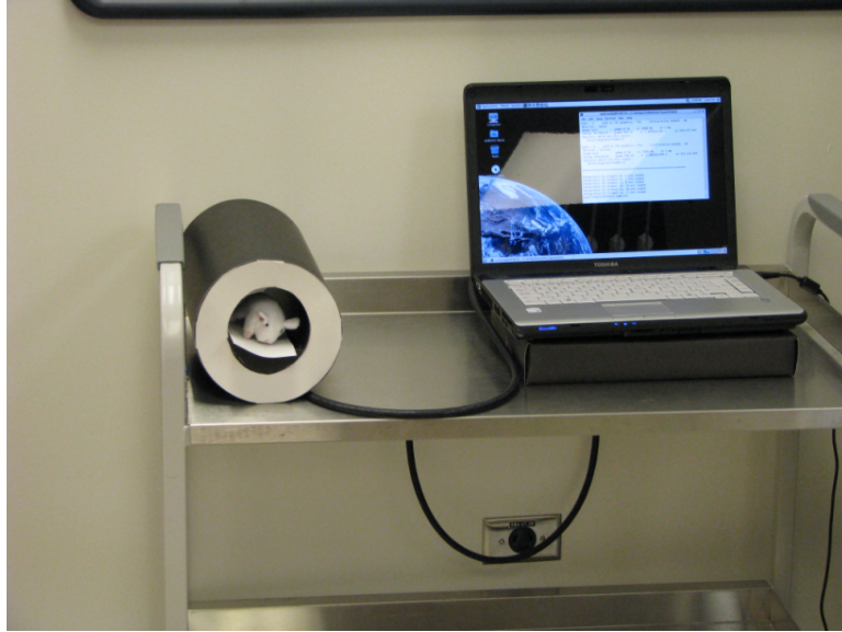
Figure 1.18: Mock-up of proposed ultra-portable PET scanner. Output from the scanner is processed by a small readout electronics system (black box), and images are stored and reconstructed on a notebook computer.
