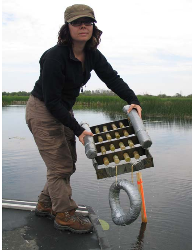
Figure 5-2: The author removing a floating NDS frame, holding 16 randomly arranged vials of four nutrient agar treatments, after its deployment in the marsh for a period of two weeks.
