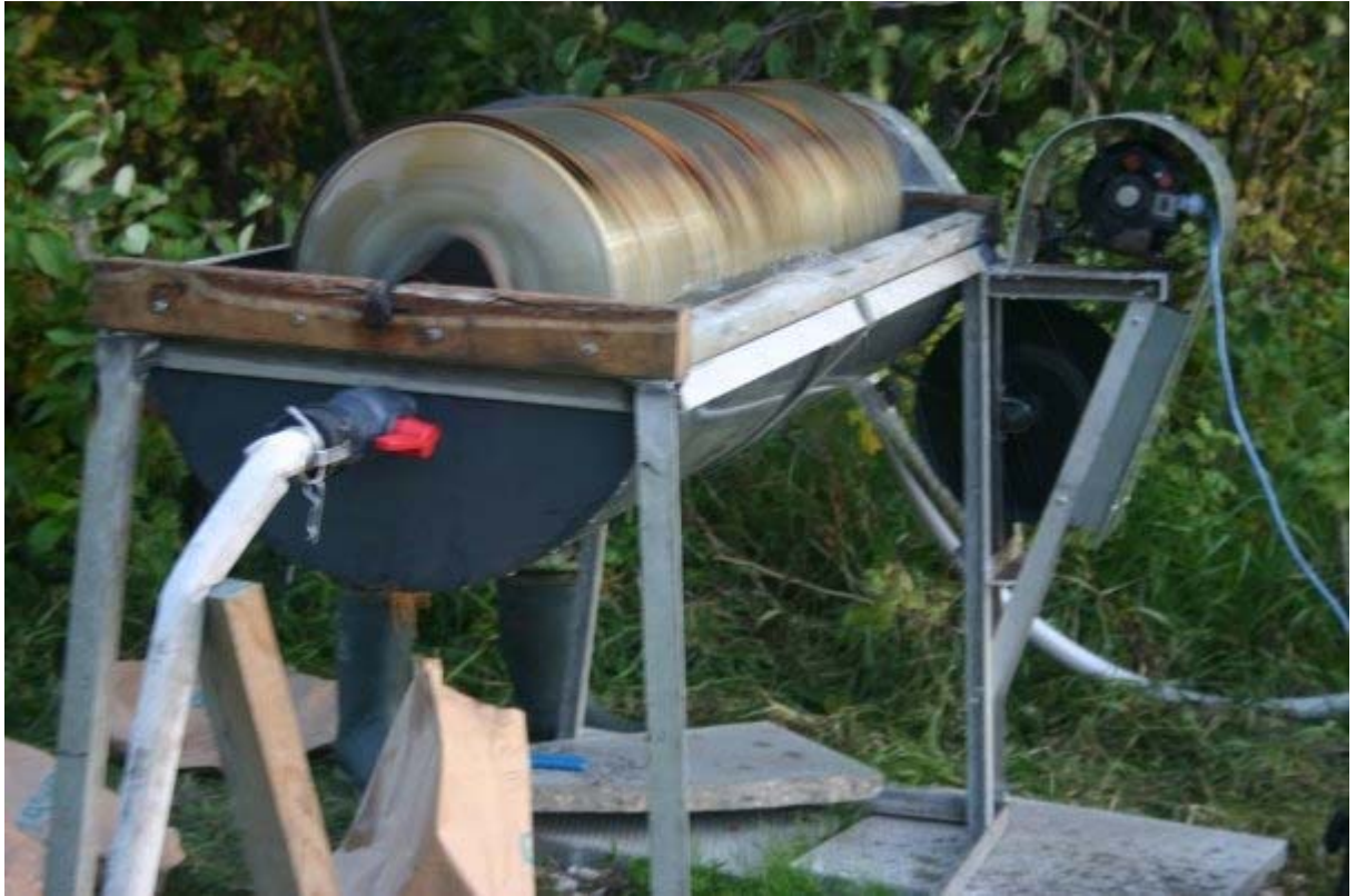
Figure 6-4: The automatic root washing machine. A submersible pump in the river forced water into the grey tub through the white hose in the foreground. An electric motor (right) caused the wire mesh cylinder to rotate. Root cores were placed in the four separate cages within the cylinder. Dirty water drained through the hose at the rear.
