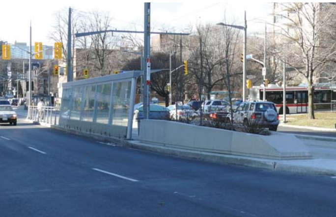
Figure 76 Planters are used at St. Clair Ave stations to direct riders to signalized intersections.
