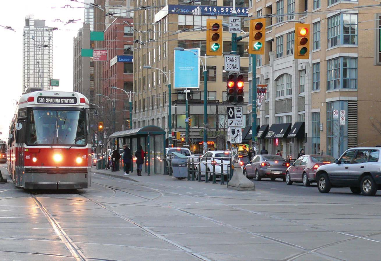
Figure 78. Spadina streetcar signals and mixed traffic lane signals.
