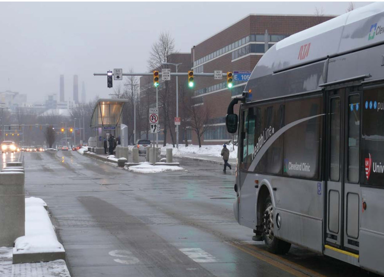
Figure 79. The Euclid Corridor uses LRT signals to avoid confusion.
