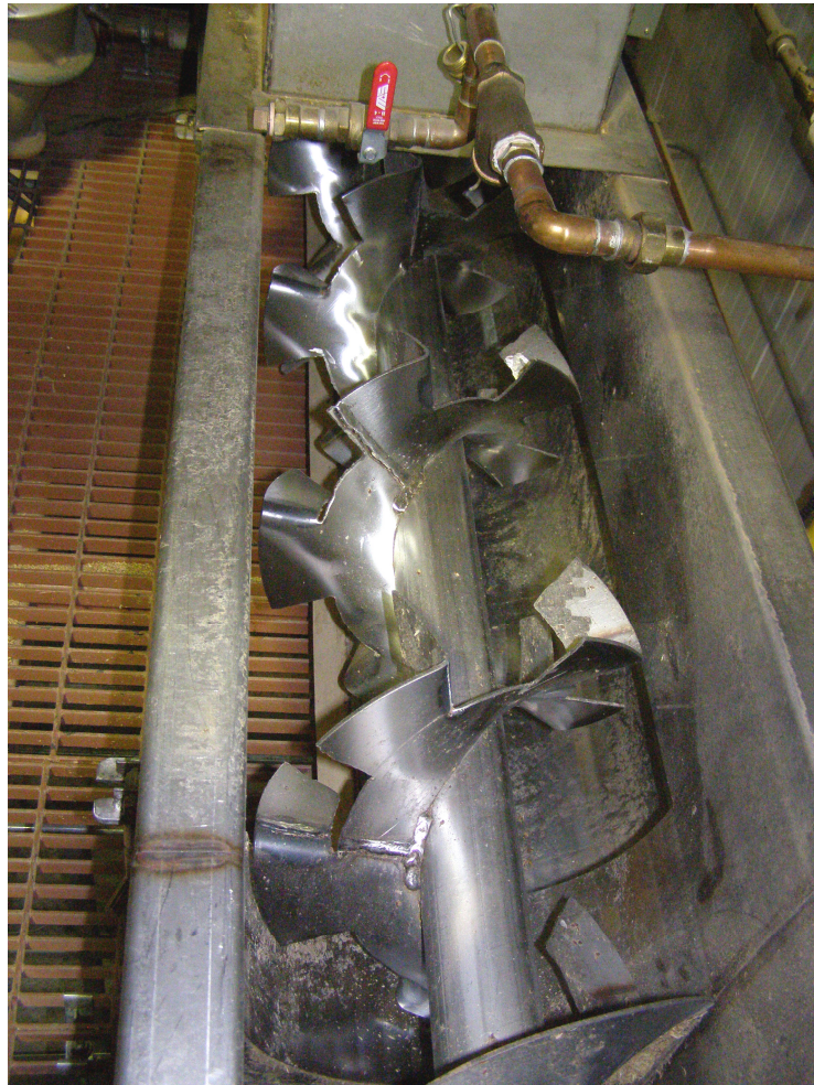
Figure 7. Grain conditioner screw conveyer with mixing paddles.
