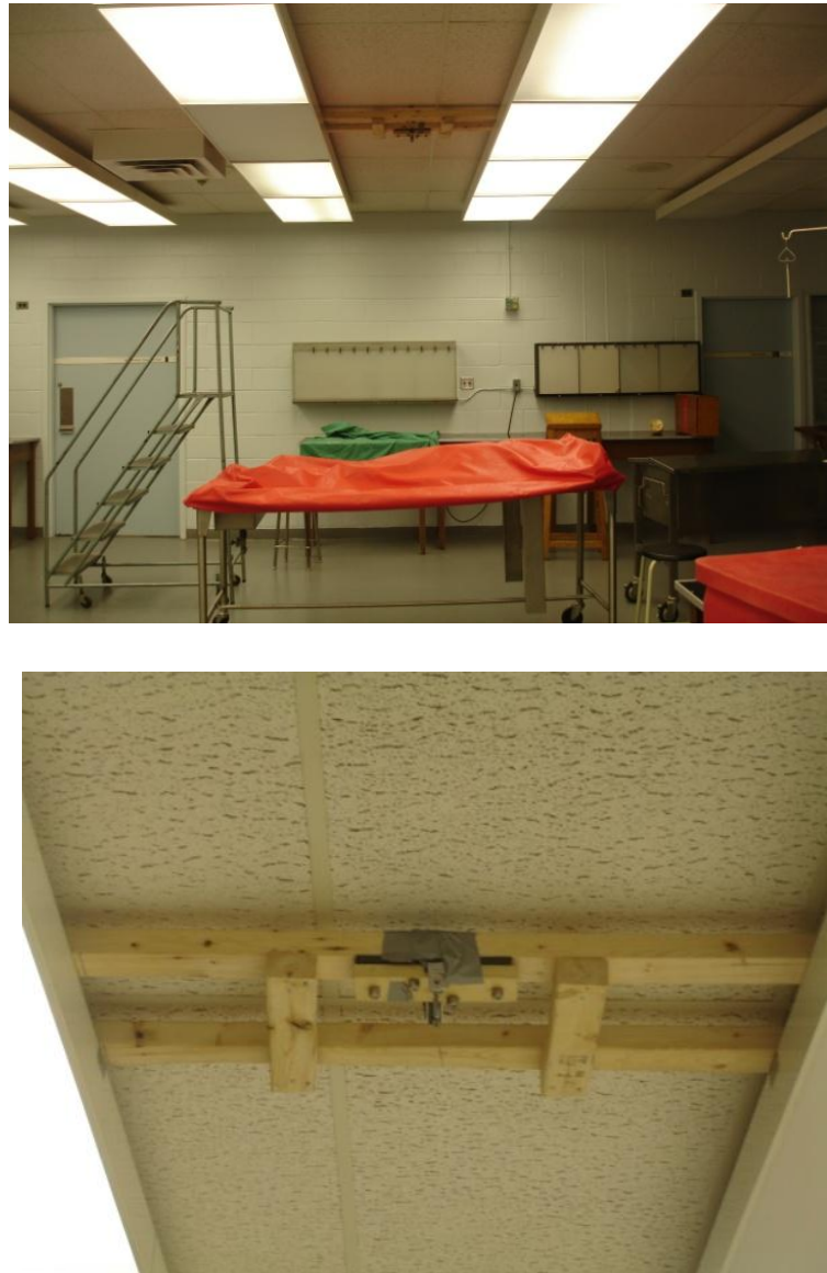
FIGURE 3- The camera mount. A) Overall view B) Close up view of mount.
