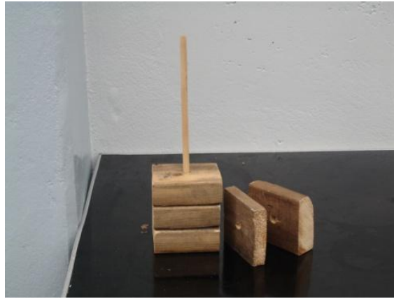
FIGURE 37- Block system separate from the setup, depicting the attached block base and the dowel fitting in the center of the blocks
