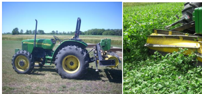
Figure 1. The blade roller (left) and the blade roller crimping a pea and oat intercrop (right).
