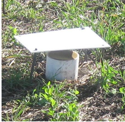
Figure 2. Polyvinyl chloride tube fitted with foam disks and a plastic canopy.
