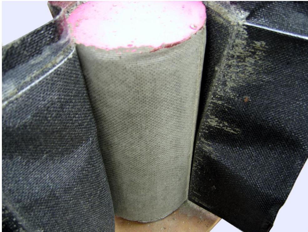
Figure 24: Stripping fabric from a fabric formed concrete cylinder
