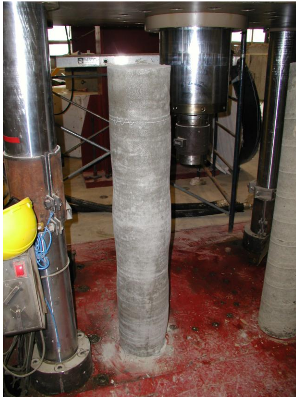
Figure 67: Bulged concrete column
