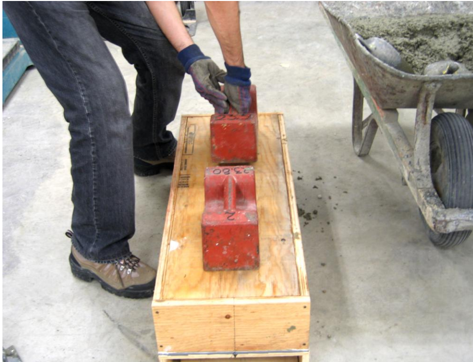
Figure 10: Extra pressure on fresh concrete to accelerate the bleeding process
