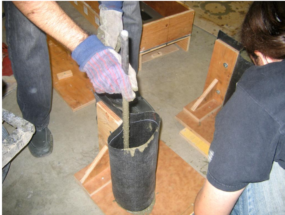
Figure 21: Compacting fresh concrete using the standard rod
