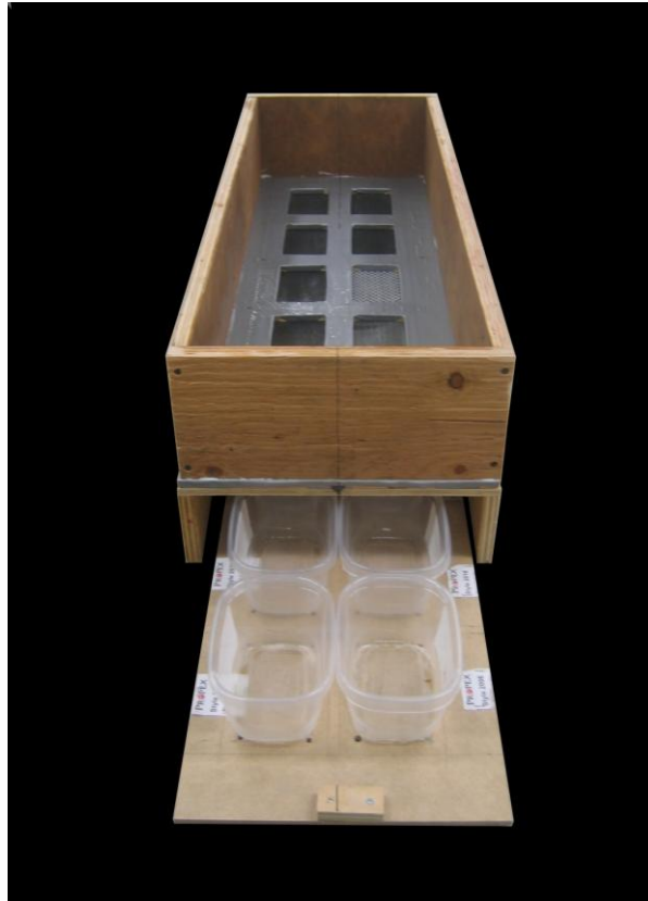
Figure 8: Box made for Box Test using normal concrete
