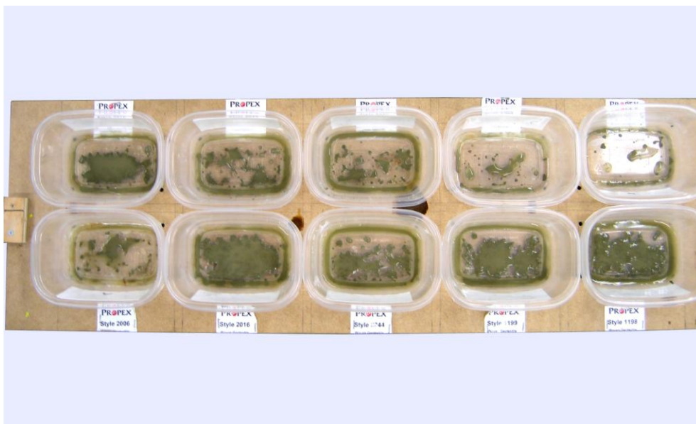
Figure 11: Collected bleed cement/water paste from fabrics tested with normal concrete in the box test
