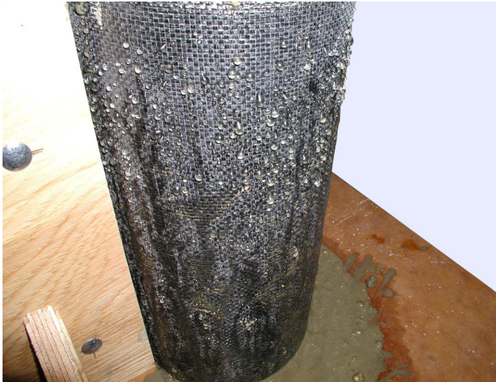
Figure 23: Bleed clear water from the walls of a 152 mm (6 in.) diameter fabric-formed concrete cylinder
