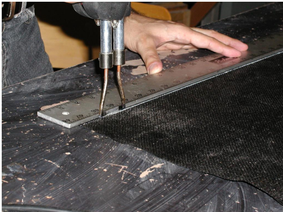
Figure 18: Soldering gun with the blade-shaped tip melting fabric and providing straight edge
