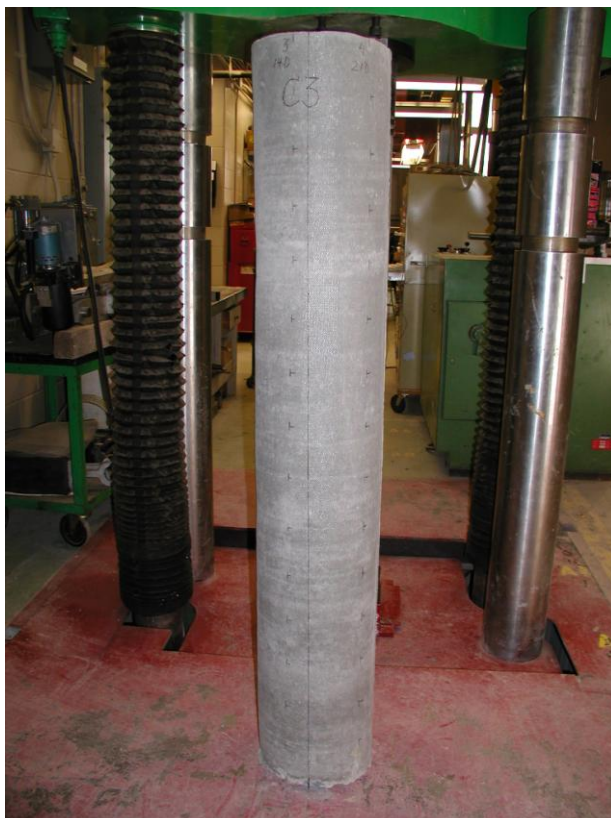
Figure 68: Modified fabric formwork resulting in a straight column
