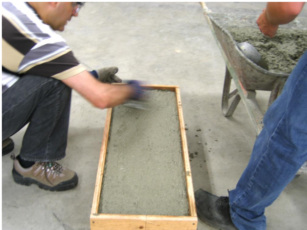
Figure 9: Filling the box with fresh concrete
