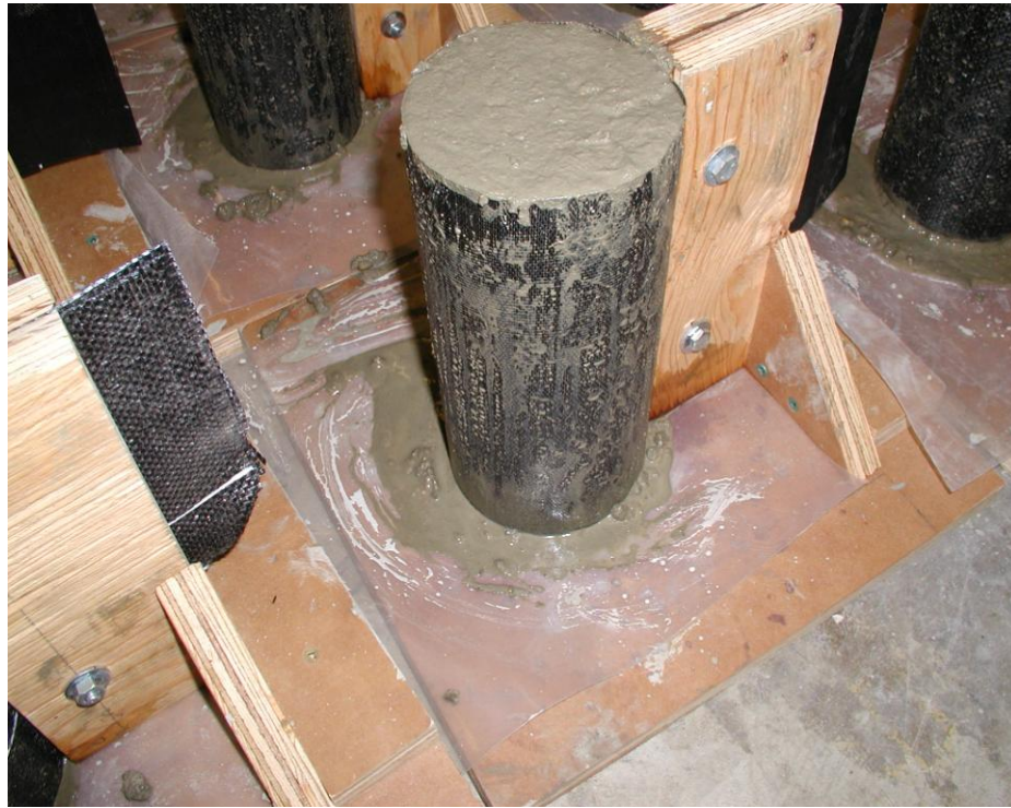
Figure 34: Fabric-formed concrete cylinders
