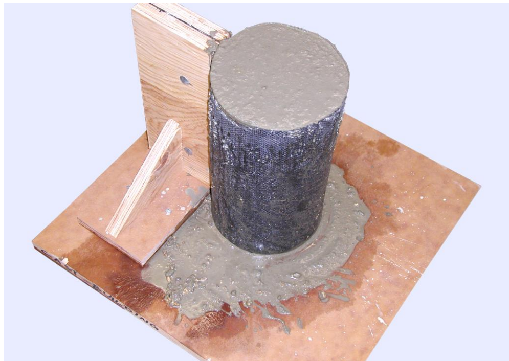
Figure 22: Fabric mold filled with fresh concrete
