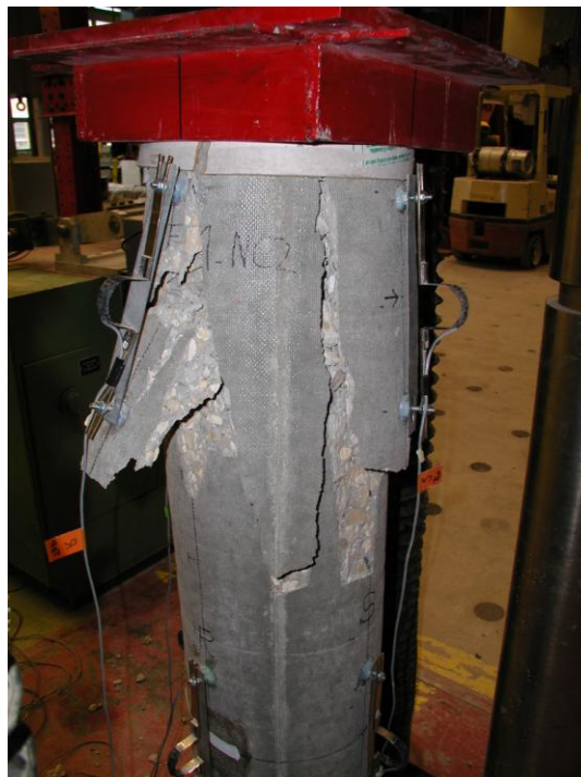
Figure 64: Column FF-NC-2 after failure
