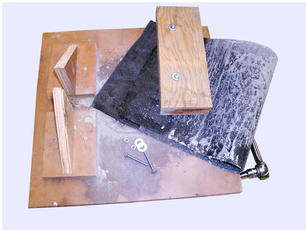
Figure 25: Reusable fabric form parts; the base, sandwich boards, bolts, and the fabric itself
