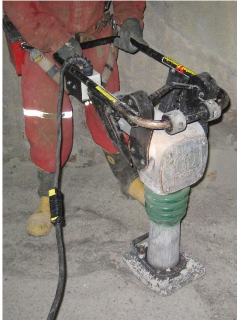
Figure 4.12: Wacker vibratory rammer compactor (AECL stock photograph)
