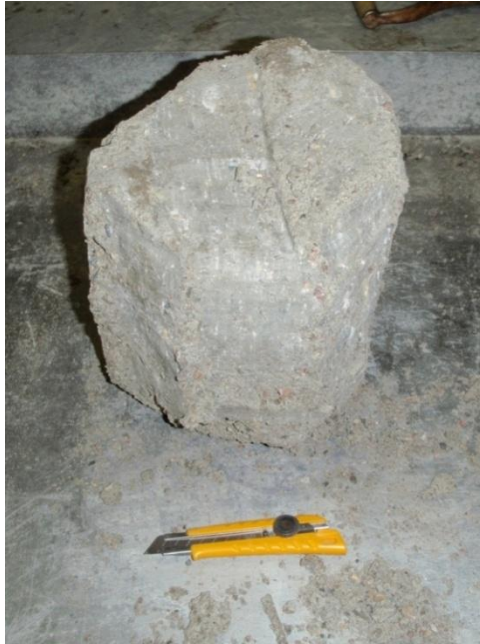
Figure 5.20: TDR calibration water content sample (AECL stock photograph)
