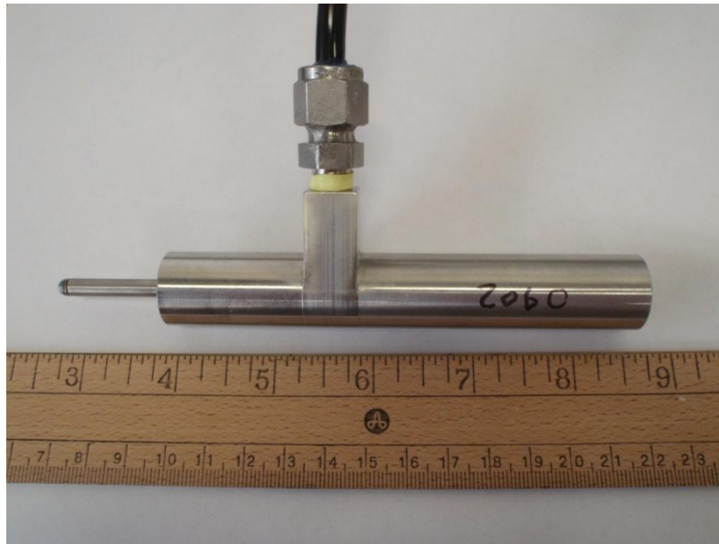
Figure 5.12: Roctest fibre optic displacement transducer model FOD-F (AECL stock photograph)
