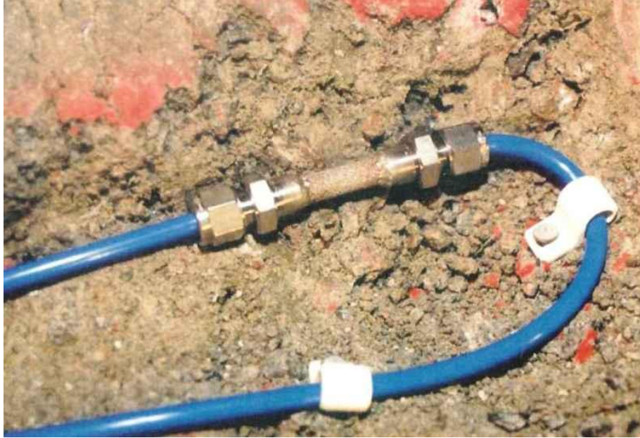
Figure 2.11: Filter tip pore-water pressure measurement in the Backfill and Plug Test (Gunnarsson, et al. 2001)
