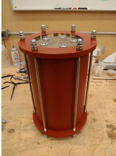
Figure 5.81: High pressure watertight TDR datalogger caisson (AECL stock photograph)
