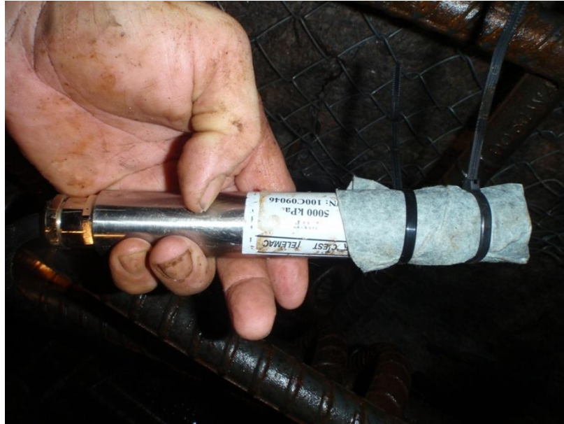
Figure 5.42: Vibrating wire piezometer filter tip wrapped with a geotextile sock (AECL stock photograph)
