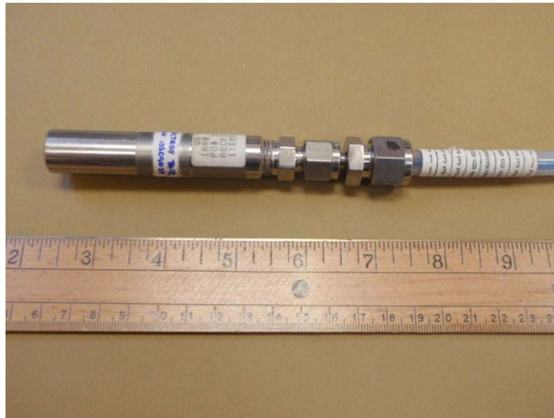
Figure 5.1: Thermocouple with stainless steel housing and Synflex cable armouring (AECL stock photograph)
