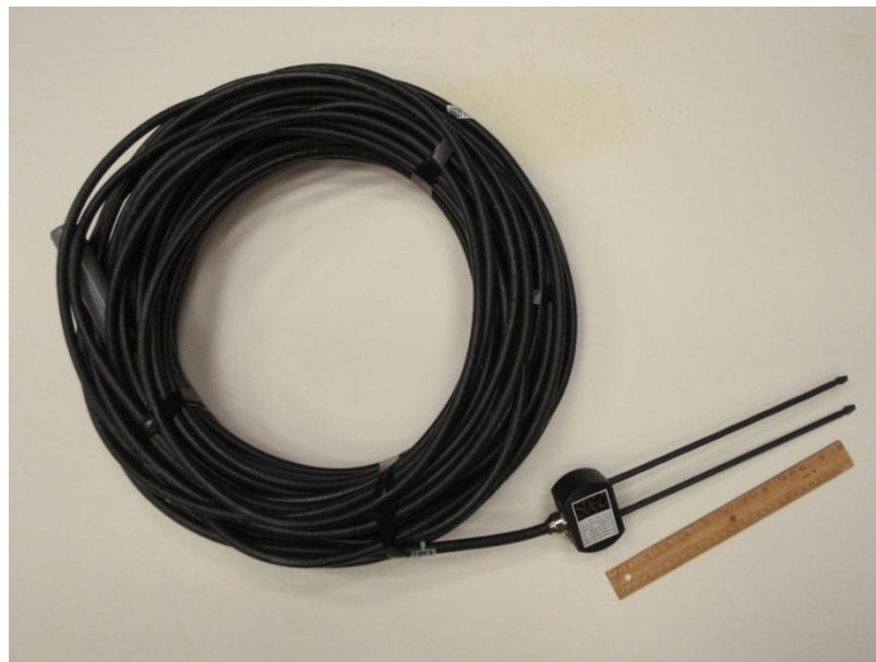
Figure 5.10: TDR probe with 50 m cable (AECL stock photograph)
