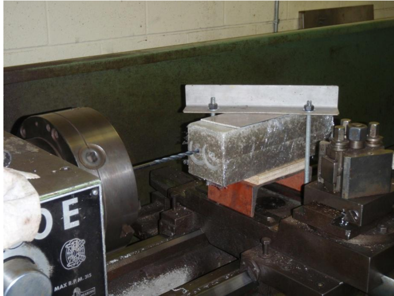
Figure 5.55: Drilling a precompacted bentonite-sand brick for TDR probe installation (AECL stock photograph)
