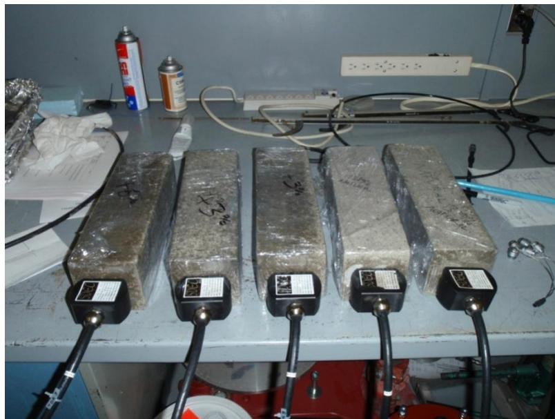
Figure 5.21: TDR probes inserted into precompact bentonite-sand bricks (AECL stock photograph)
