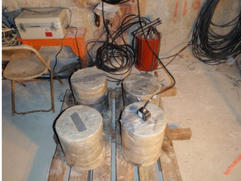
Figure 5.18: TDR probe inserted into a bentonite-sand cylinder for calibration (AECL stock photograph)
