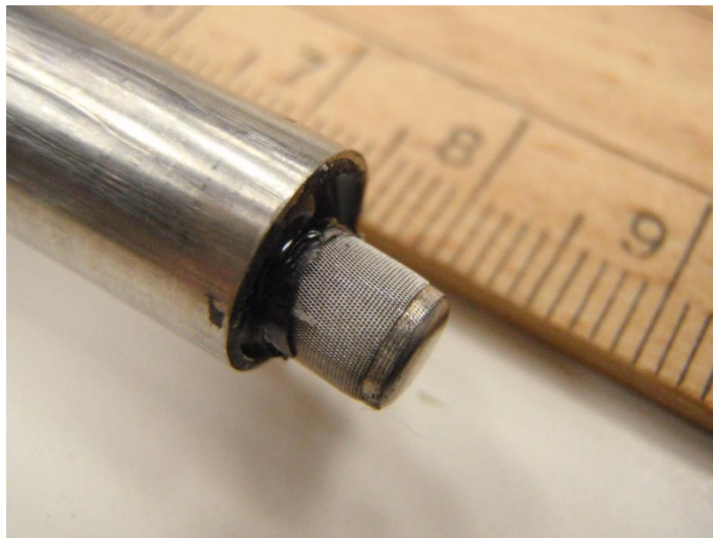
Figure 5.23: Psychrometer tip waterproofing and armoring (AECL stock photograph)
