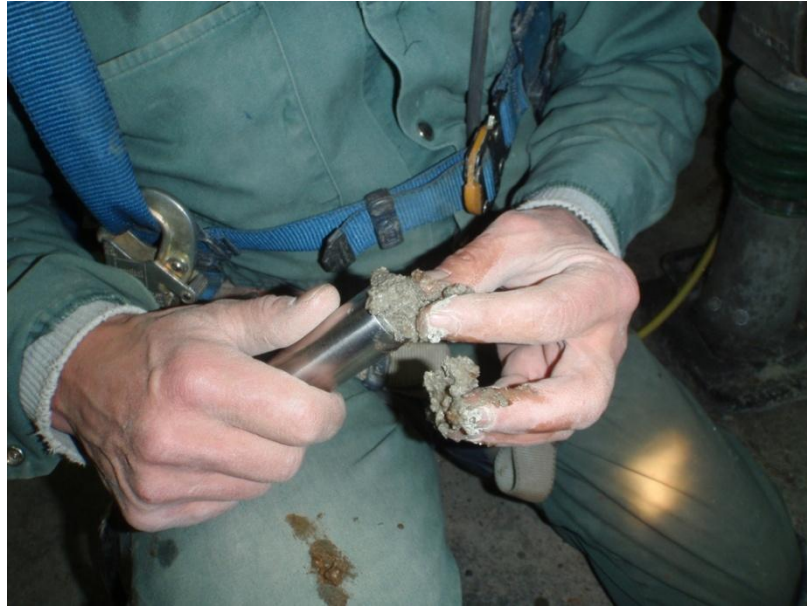
Figure 5.46: Smearing filter of a piezometer with saturated bentonite-sand material before installation (AECL stock photograph)
