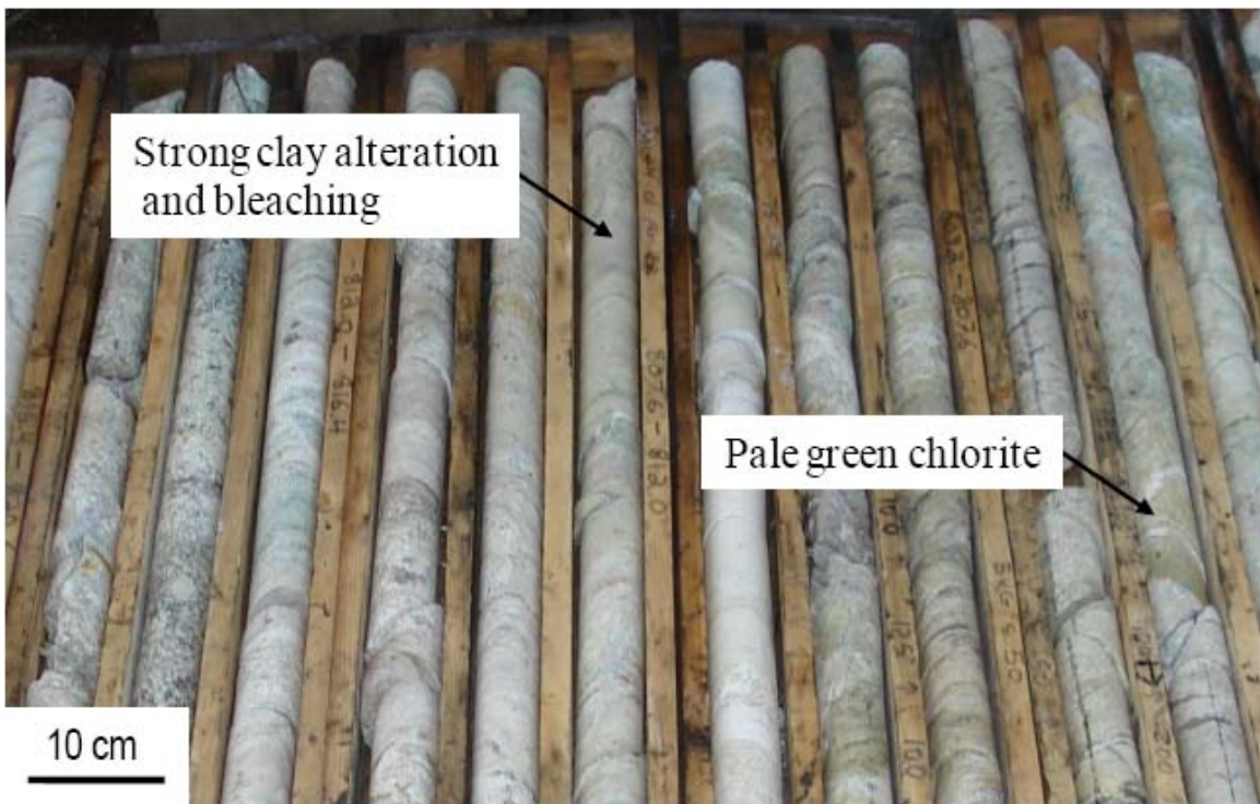
Figure 4.4: Drill core image showing strongly bleached and clay altered pelitic – psammopelitic gneisses and pegmatite units in proximity of reverse fault. Note pale green chloritization CX-44-1 799.5 - 815.5 m (Increasing depth from right to left).
