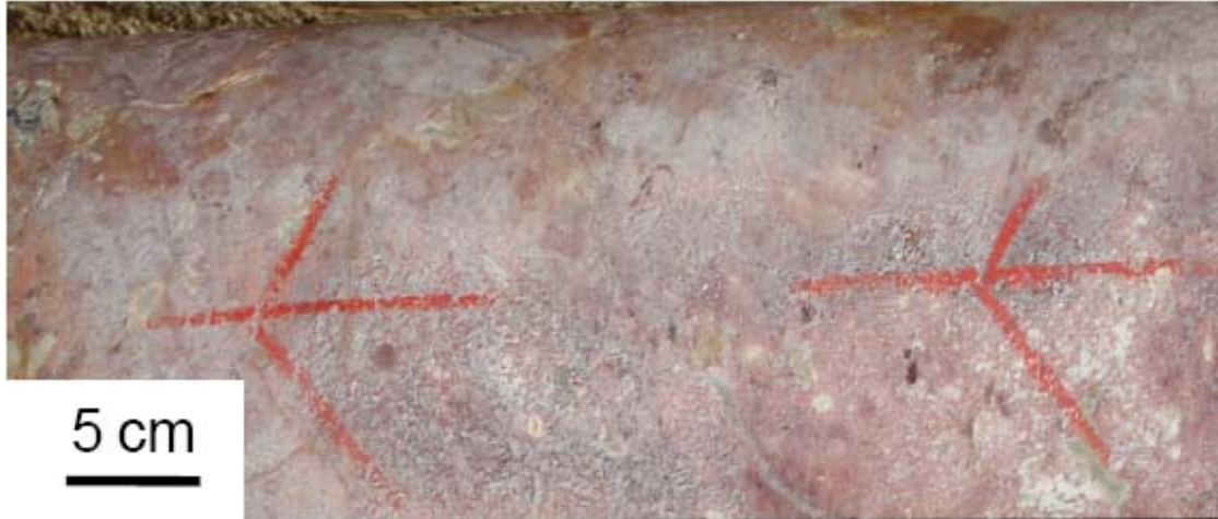
Figure 4.5: Drill core image showing secondary hematite overprinted by late clay alteration and bleaching of psammopelitic schist DDH CX-51-1 737.5 m.
