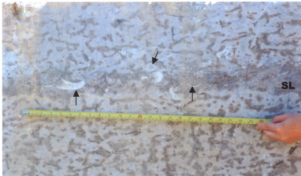
Fig. 1.1: Tyndall Stone section with typical mottling. Fossils (shown by arrows) occur commonly within storm lenses (SL).
