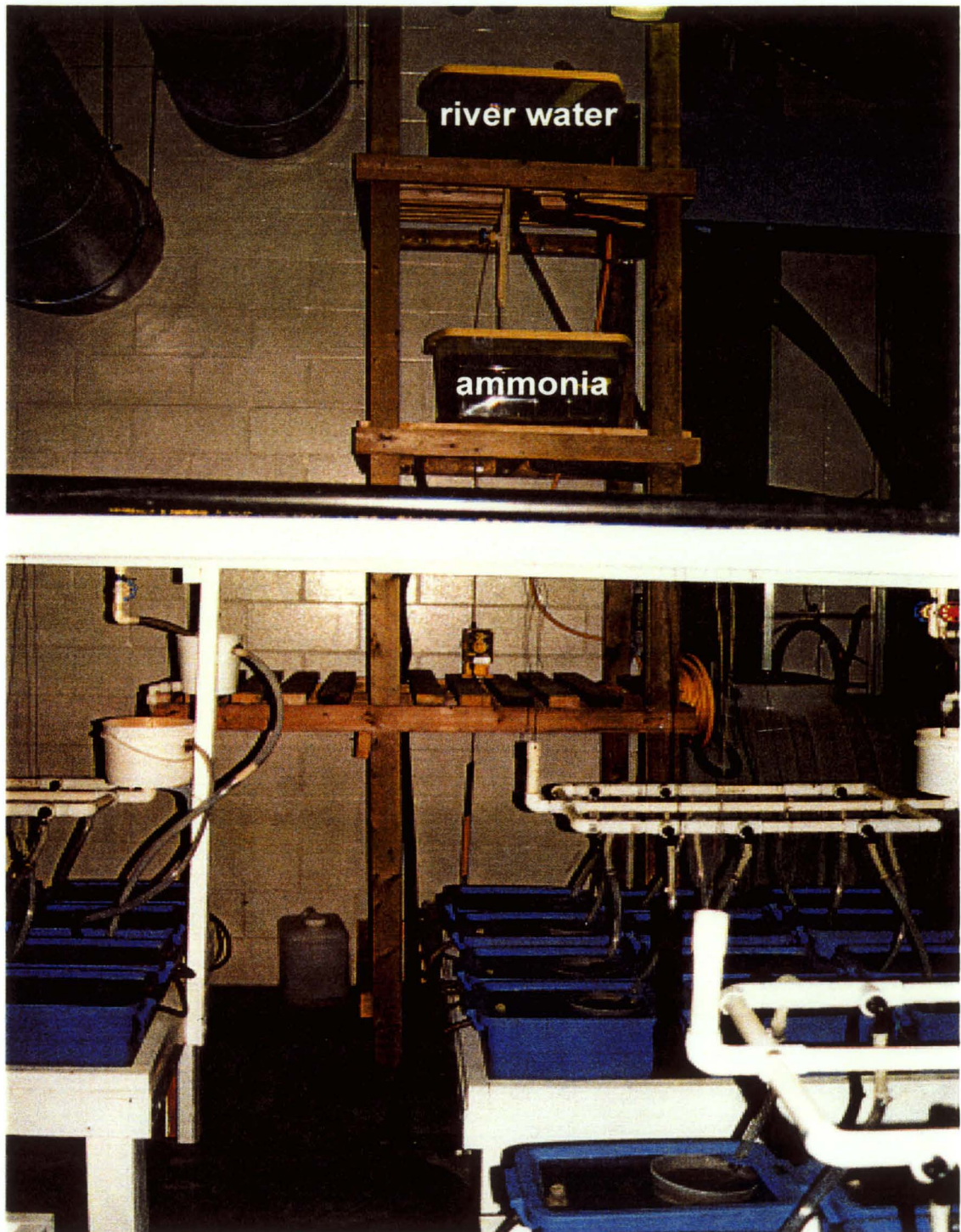
Figure 4-10. Shelving unit with river water and ammonia supplies.
