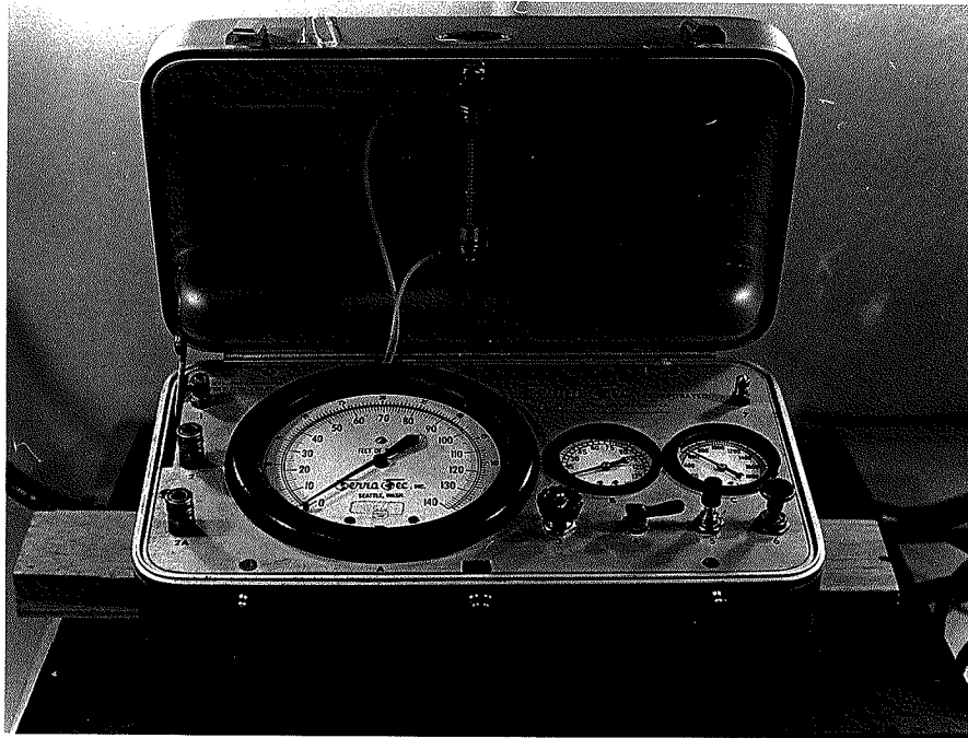
Figure 4 - Portable Control Box For Air-Activated Piezometers
