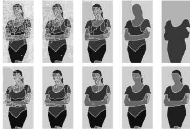
Figure 2.9: Results of scale-space watershed segmentation using Gaussian diffusion (Top) and CLMC (Bottom) to reduce over-segmentation. Images from [5].
