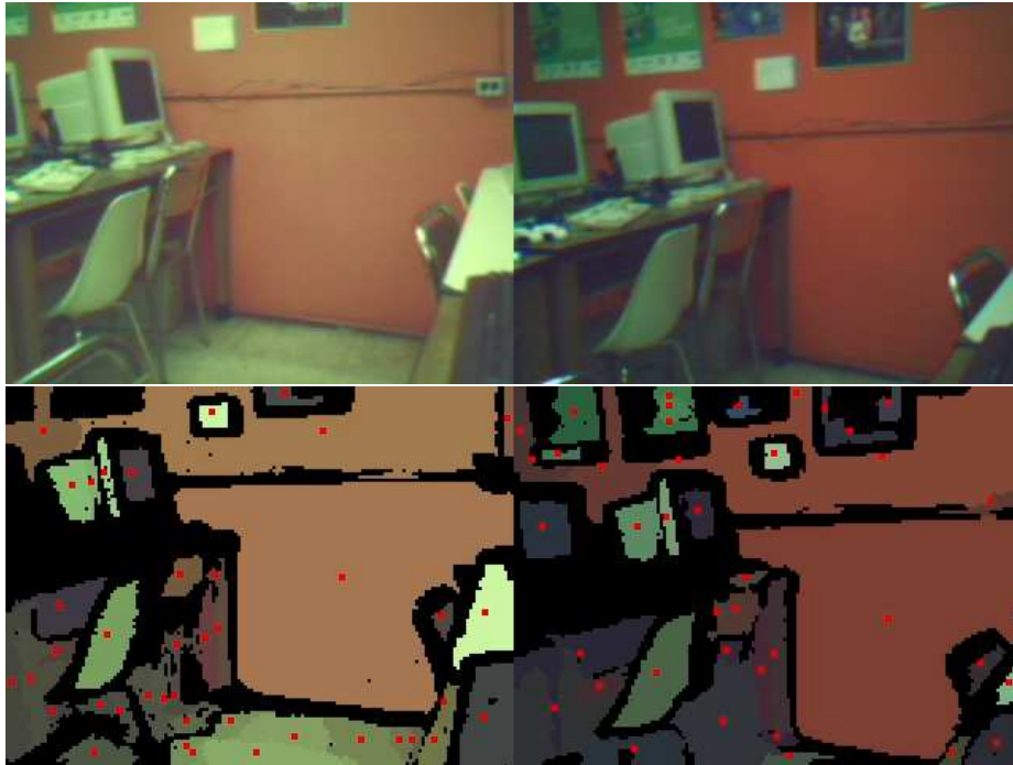
Figure 2.10: The region segmentation (bottom) is produced from the raw image (top). The dot inside the regions represent the centroid point. Images from [6].
