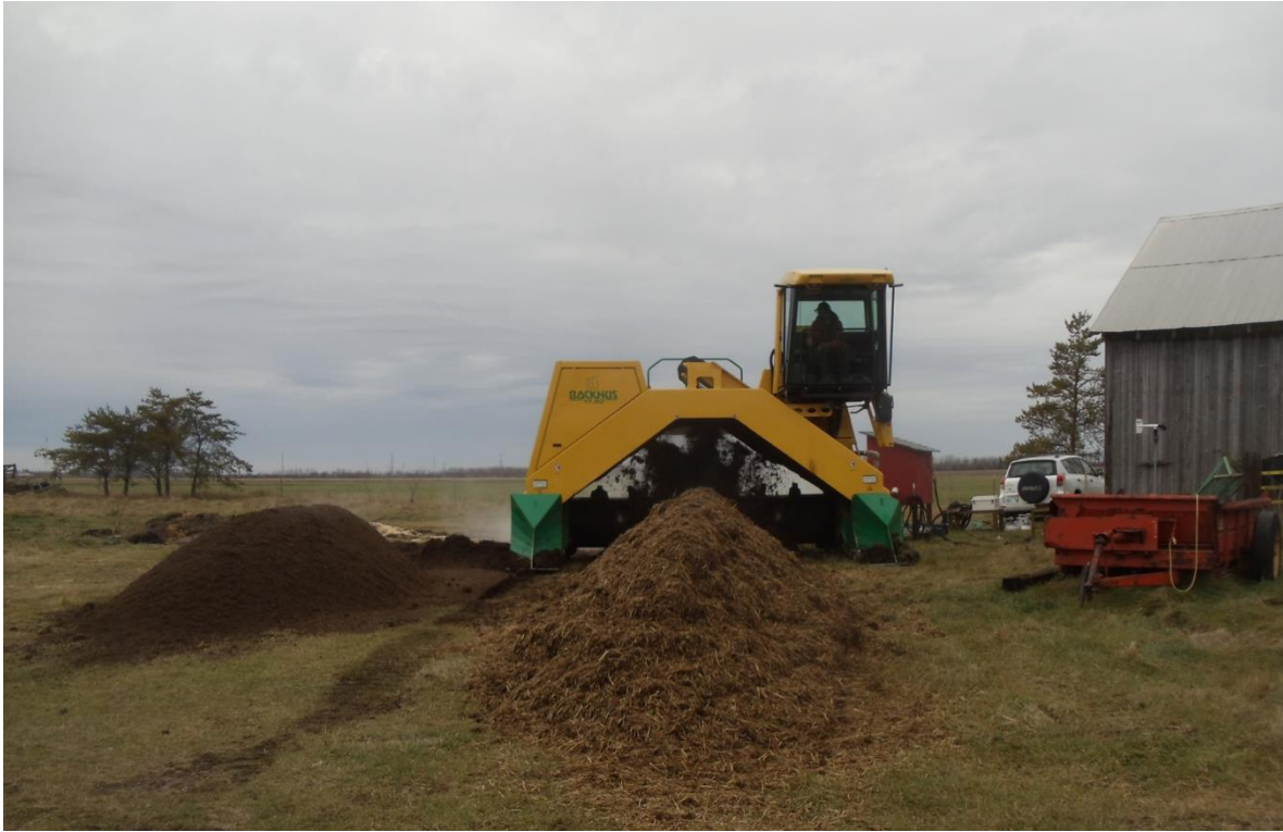
Figure 4.1 Turning the windrows with a Backhus windrow turner on October 22, 2011 (DOY 296).
