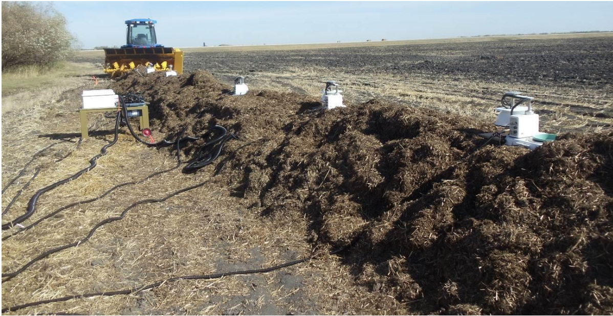
Figure 3.1 Trial 1 windrow, prior to turning on September 21, 2011 (DOY 263), with automated chambers set up, as well as Brown Bear windrow compost turner in background.
