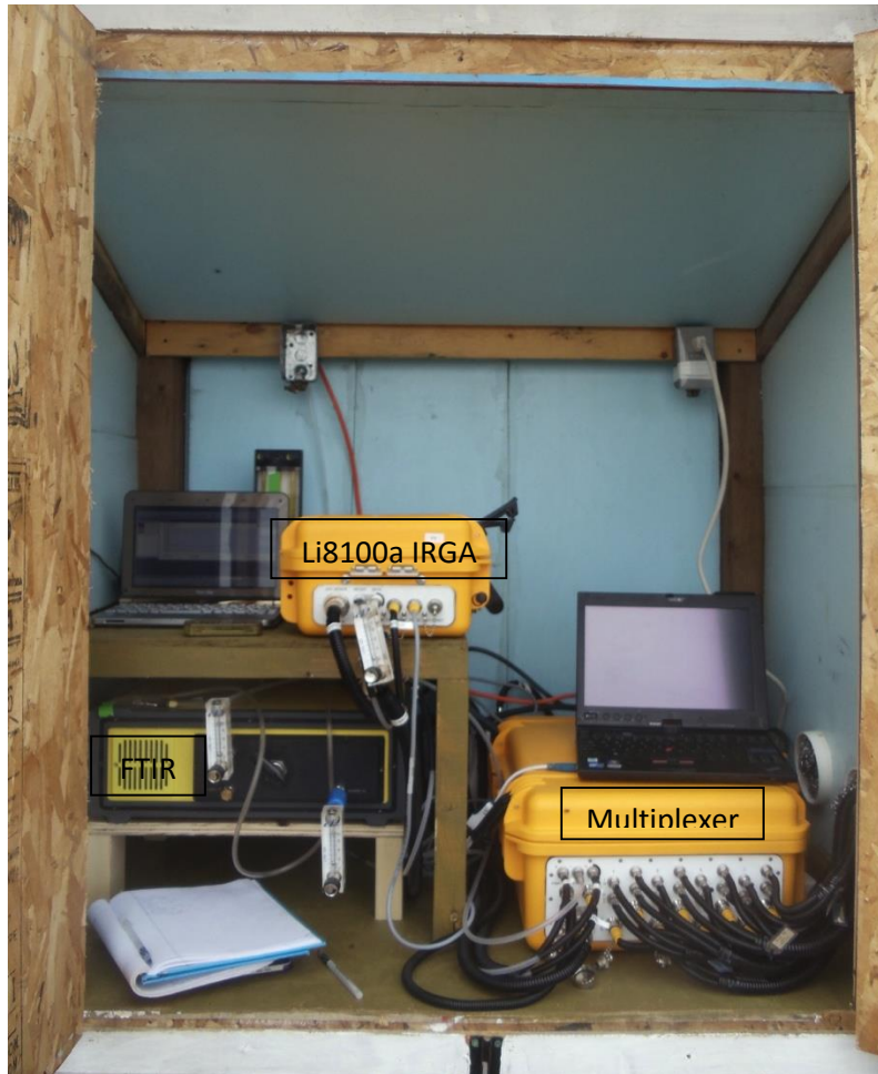
Figure 2.1 Setup of the multiplexer, Li8100a IRGA, FTIR, and data recording laptops in insulated storage unit. Büchner flask installed after the photo was taken.
