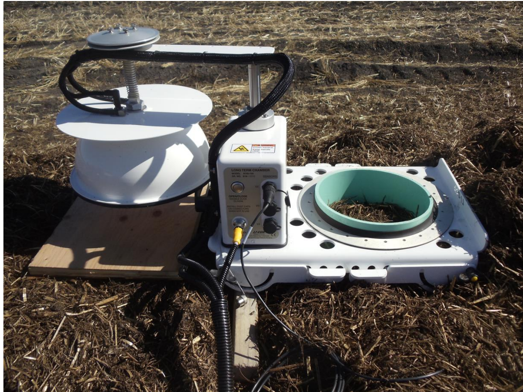
Figure 2.2 Automated chamber, in open position, setup on the peak of a compost windrow.
