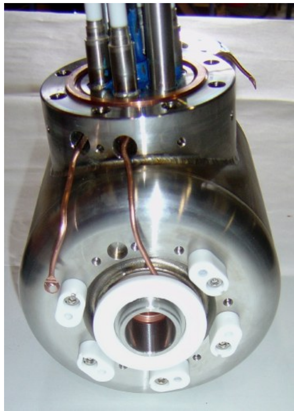
Figure B.4: The collector head during assembly. Note that the copper seal visible is a custom size due to required geometry. For dimensions see Figure B.1.
