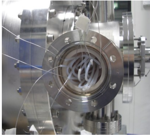
Figure 3.19: Photo of the folded electrode wires in the ceramic insulators. With the magnet and trap located to the left, half of the electrode wires can be seen before they were cut and attached to the electrical feedthrough flange.
