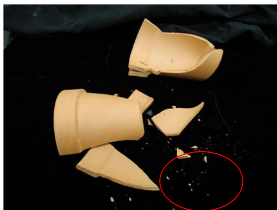
Figure 3.6: Five broken pieces of the flowerpot. The red circle highlights debris that was too small to be effectively scanned.
