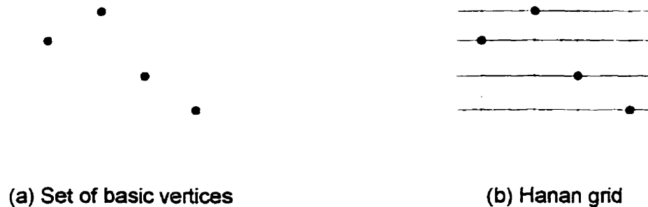
Figure 2-1: Basic vertices and Hanan grid
