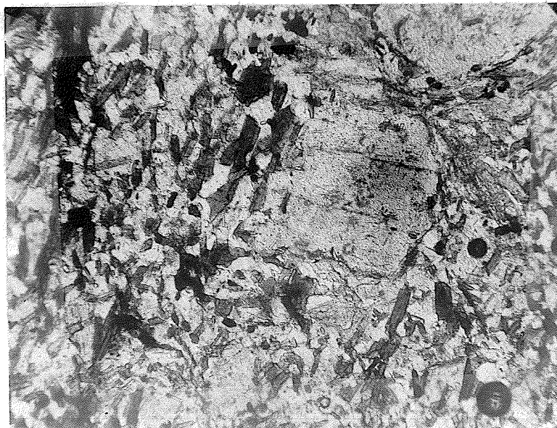
B. Biotite schists showing "phenocrysts" of plagioclase developed by metasomatic replacement. Ordinary light. X80. (Specimen N-33-3)
