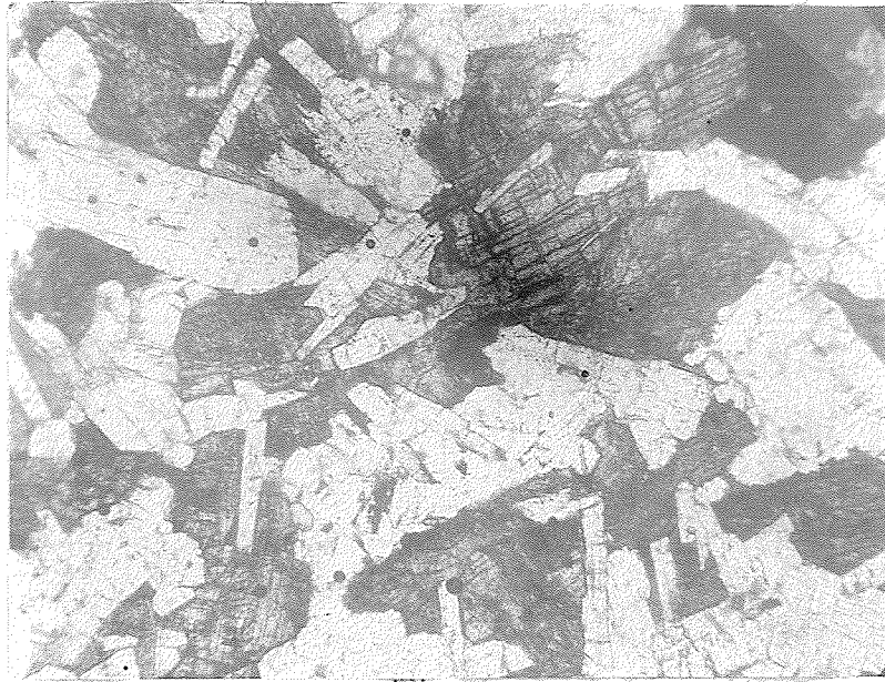
A. Medium-grained diabase showing typical. Ordinary light. X25 (Specimen FN-1-1)
