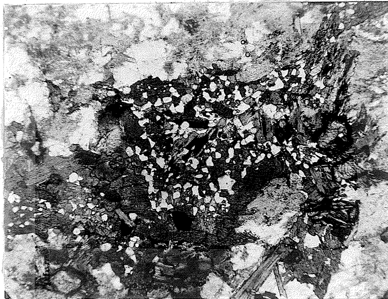
B. Basic phase of the Shenston-Mather intrusion showing the poikilitic habit of the hornblende. Ordinary light. X25 (Specimen F-7-6)
