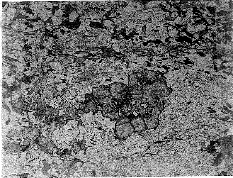
A. Biotite schists showing porphyroblastic garnet and clots of chlorite and muscovite. Ordinary light. X25. (Specimen N-12-7)
