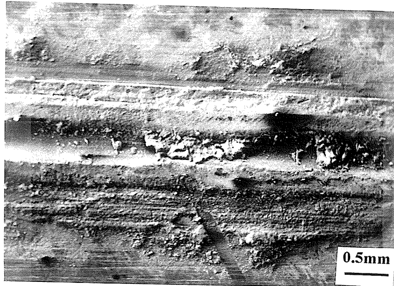
Fig.4.15 The surface appearance of a low-g weld showing the oxidation around the weld due to insufficient shielding of argon gas.
