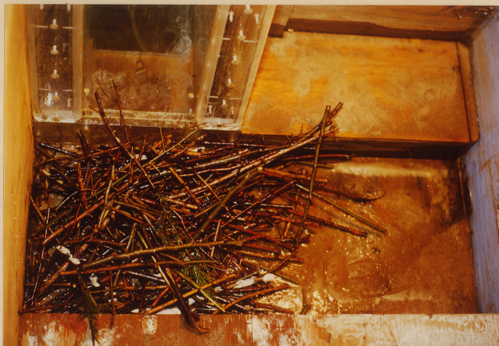
Plate 8 Orifice Spillway Flume Model Saturated Trash Tests - Before
