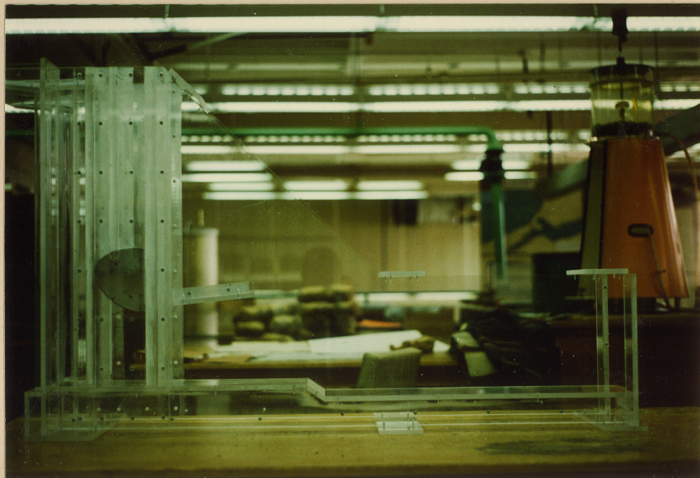
Plate 2 Overflow Spillway Flume Model - Diversion Configuration
