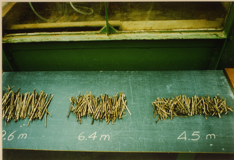
Plate 7 Dry Trash for the Comprehensive Model Trash Tests Approximate prototype lengths: 9.6 metres, 6.4 metres, 4.5 metres
