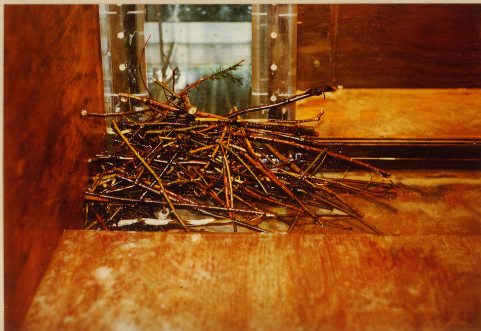
Plate 9 Orifice Spillway Flume Model Saturated Trash Test - After
