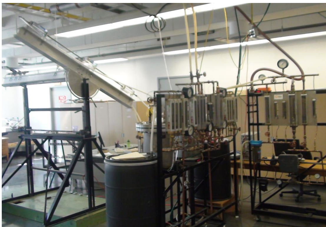
Fig. 3.3 Test loop with an inclined junction
