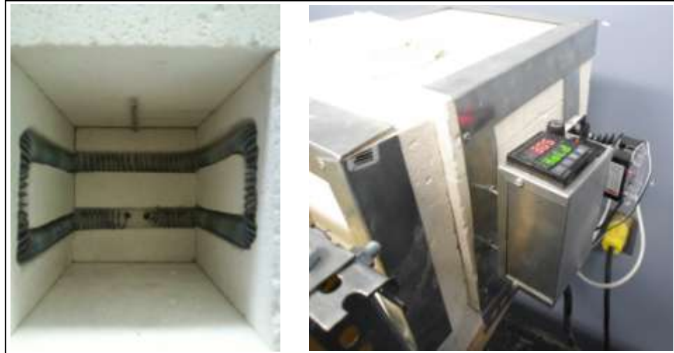
Figure 3.4: Furnace interior (left) and exterior, showing control box (right)
