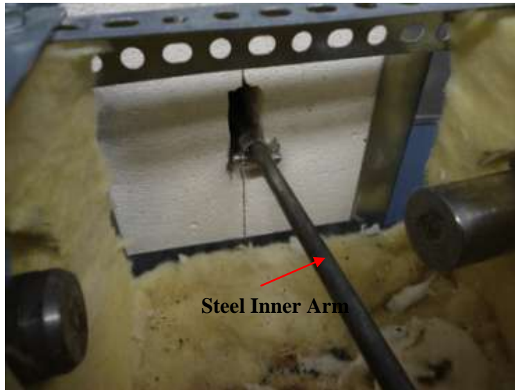
Figure 3.13: High temperature fixture (heating position with specimen in furnace for heating)
