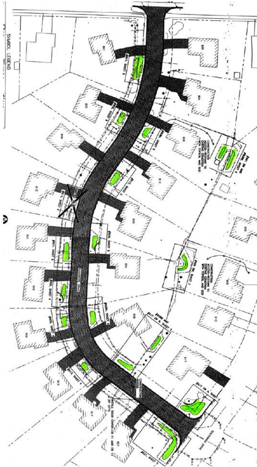
Figure 4.1 Treatment Watershed Rain Garden Layout in Burnsville (Barr, 2006)
