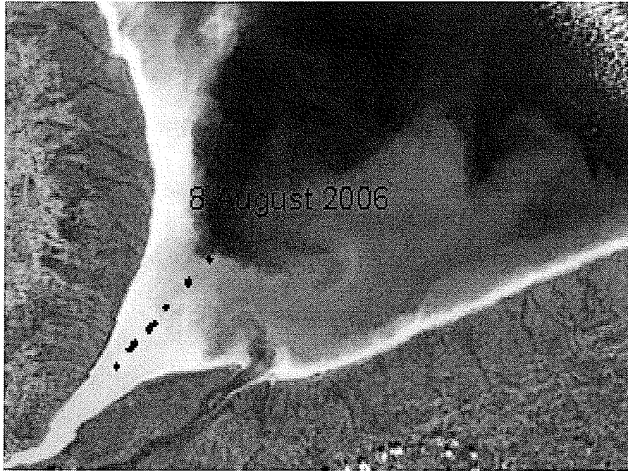
Figure V.23; MODIS image showing CTD measurements transect for the Nelson River estuary for 8 August 2006
