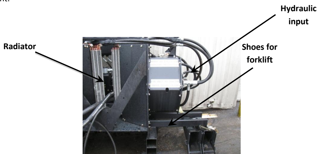
Figure 1. The load simulator presently used at MacDon [1].
