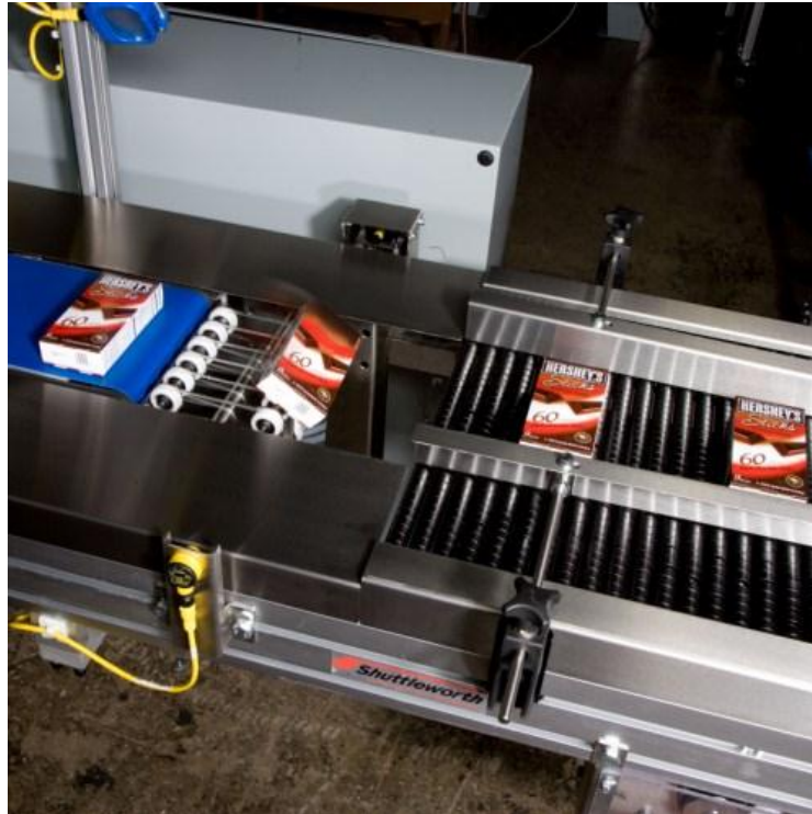
Figure 33. Shuttleworth rejection system that uses a retractable mechanism allowing the rejected to fall below as shown here [17] (Used by permission of Shuttleworth, LLC)
