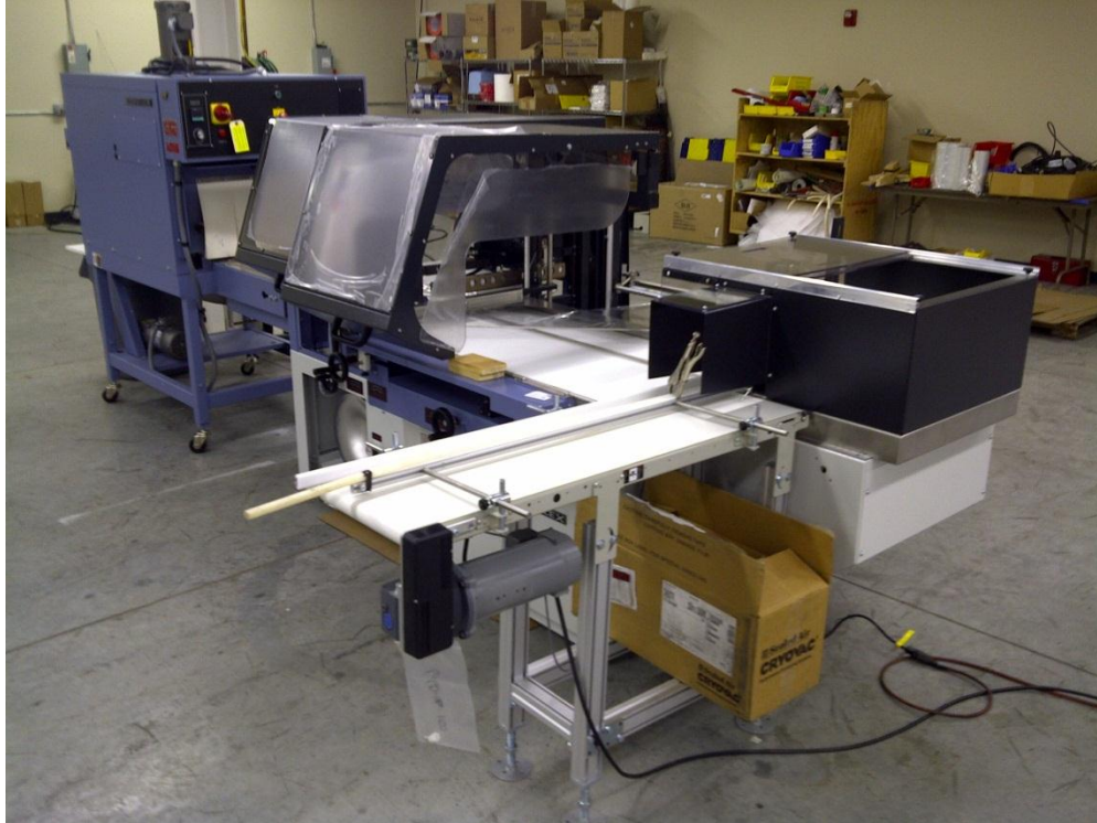
Figure 3. Output of the check weighing cell placed on the input conveyor (lower left) of the Conflex tiling machine [3] (Used by permission of The Royal Canadian Mint).
