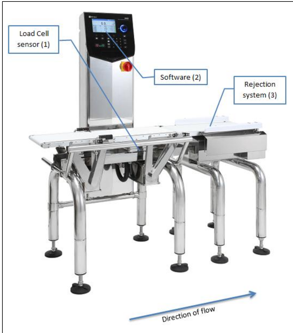
Figure 23. Ishida DASC-G-S015-12-SS check weigher components [16] (Used by permission of Ishida).
