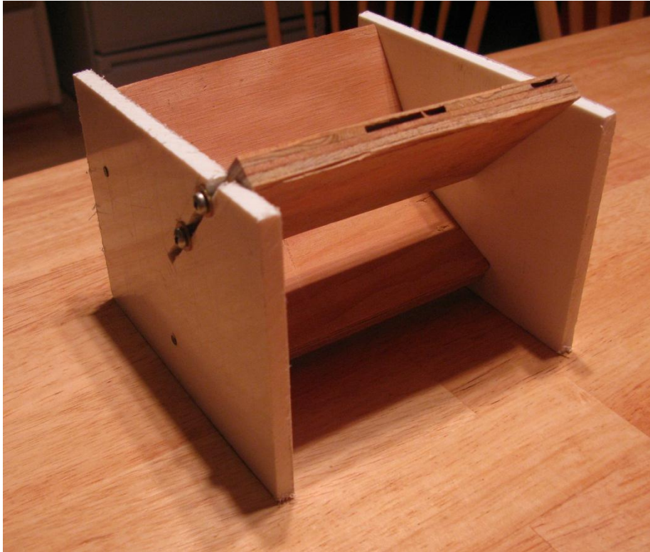
Figure 40. Roll transfer mechanism used for transferring coin rolls onto the tiling conveyor
