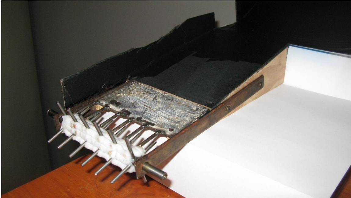
Figure 39. Buffer ramp and drop mechanism used to drop single rolls onto the main conveyor
