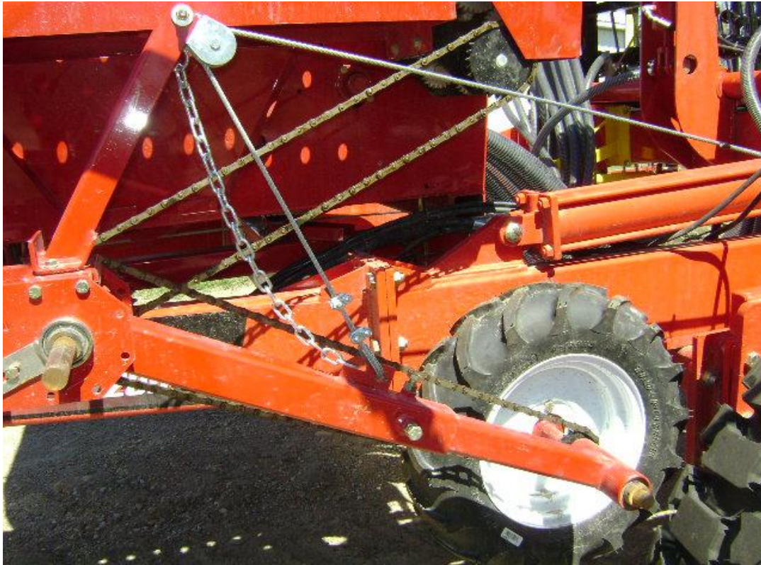
Figure 3. Current metering drive system [4]. Photo used with permission from Valmar.
