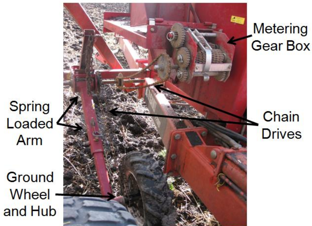
Figure 4. Current metering chain drive design. Photo credit: Rob McDougall.
