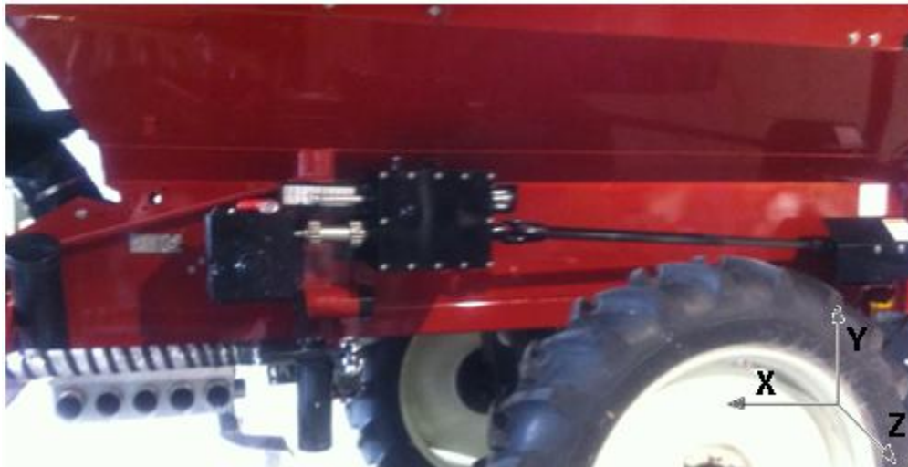
Figure 4 - Diagram of Gearbox Configuration Showing the Direction of Allowable Changes. [1]
