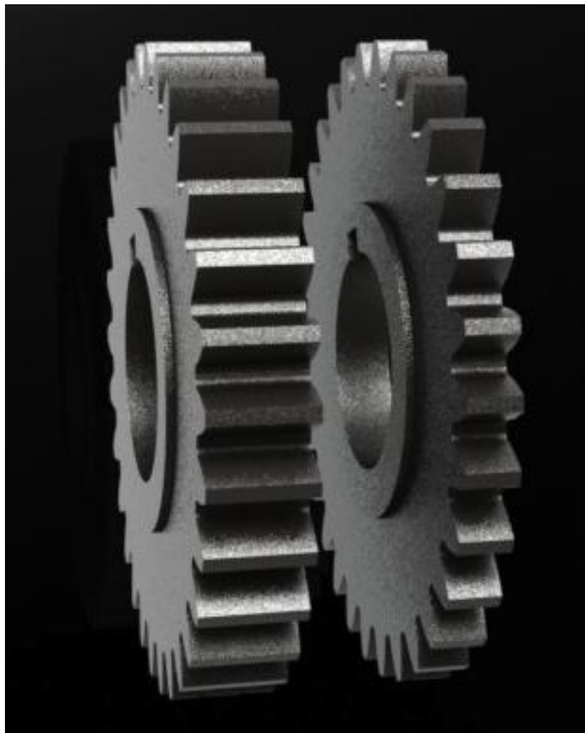
Figure 13 - Gear Size Difference From Current Gear Design (left) to Improved Design (right).
