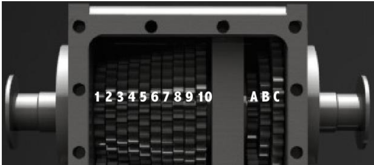
Figure 5 - Current Gear Configuration Labeled A-C and 1-10 with A and 1 Being the Smallest Gears.
