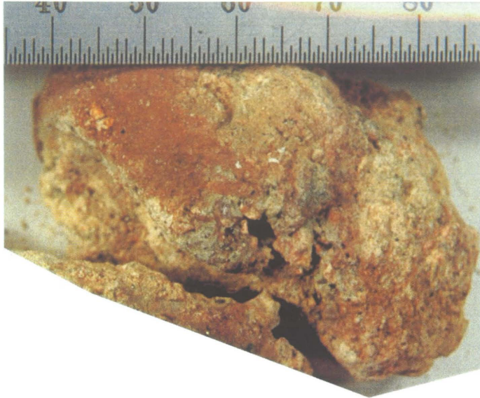
Figure 7: Example of friable, clay-bearing rubble from highly altered granite core sample from Borehole URL-7.
