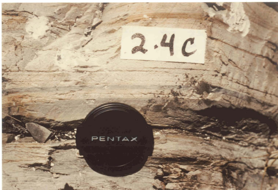
Figure 20: Photograph of multiple, light brown to brownish grey, normally graded beds in flow unit 1a in the lower ignimbrite (Member 1). Note the presence of inter-laminated, light grey and dark grey tuff at the top of the graded bed in the central part of the figure. Lens cap for scale is 5.5 cm in diameter.
