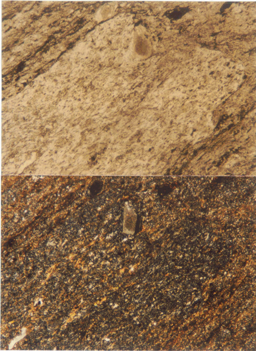
Figure 4: Photomicrographs (plane light, above and x-polars, below) showing an elongate, plagioclase-phyric dacite fragment (beige in plane light, grey in x-polars) composed largely of plagioclase and quartz with minor carbonate, sericite, and pyrrhotite. The texturally similar, fine-grained, quartzo-feldspathic aggregate surrounding the dacite fragment is inferred to be recrystallized vitric ash. The dacite fragment is from the upper ignimbrite (Member 7).
