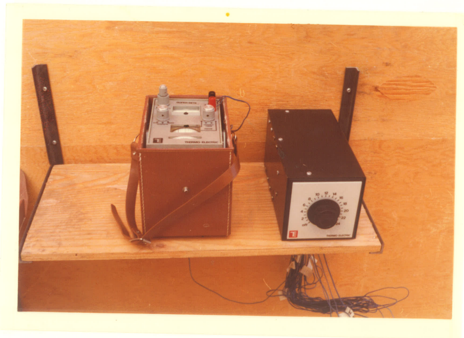
FIGURE 4-3 Temperature Measurement Using the Portable Potentiometer and Thermocouples
