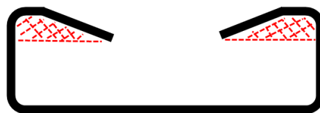
Figure 10 - Concept sketch of automobile tire showing void at upper sidewall region, as indicated by red dashed lines.
