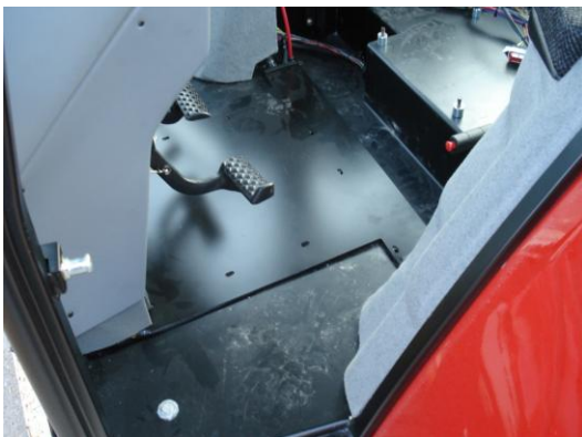
Figure 9 - Image of cab with floor plate installed
