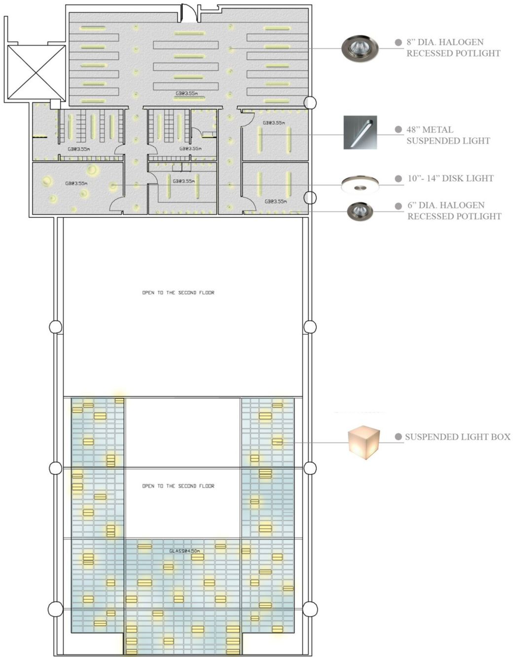
Figure 54: First Floor Reflected Ceiling Plan
