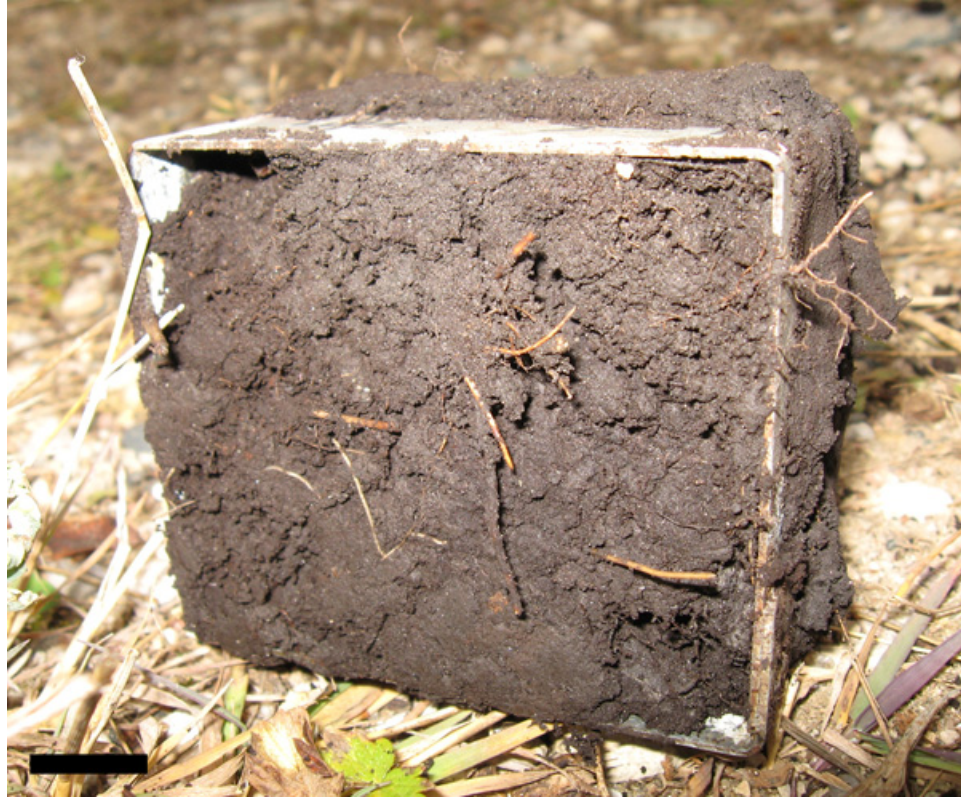
Figure 3.3. A 250 mL Kubiena box containing soil sampled from a site 1 soil profile at a depth of 15 cm. The Kubiena box would then be trimmed to remove excess soil and the soil was collected for bulk density analysis. Scale bar = 1 cm.
