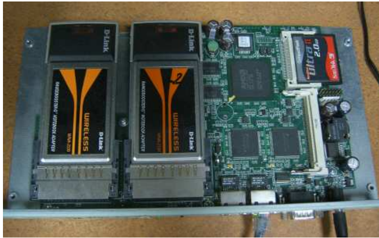
Figure 4.7: Our testbed node: A net4521 Soekris board [148] with two IEEE 802.11b/g Dlink-WNA2330 interfaces [150].
